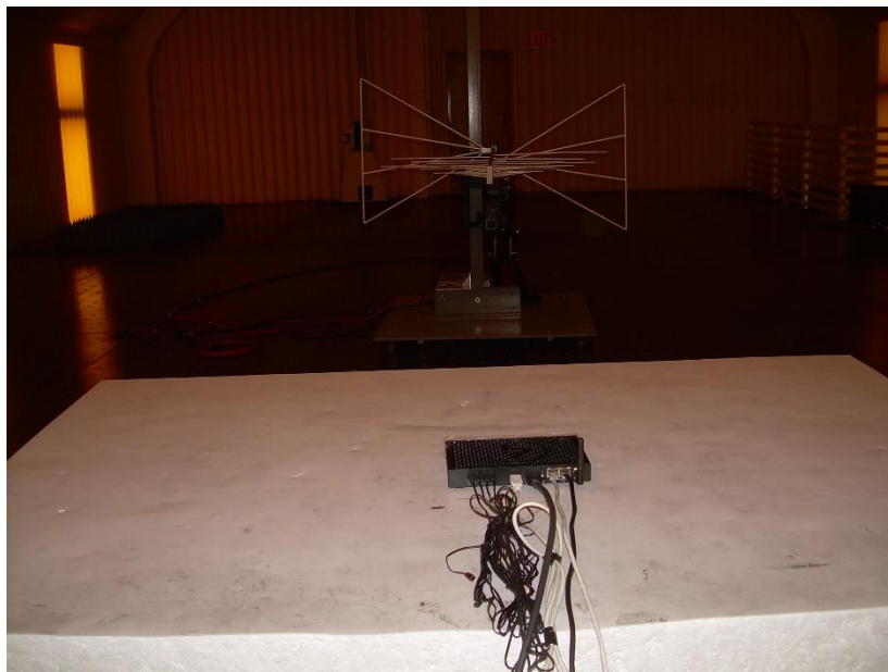
Photograph 2: Back View Radiated Emissions 30 MHz – 1000 MHz Configuration
