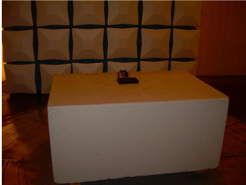
Photograph 1: Front View Radiated Emissions Below 1000 MHz Configuration
