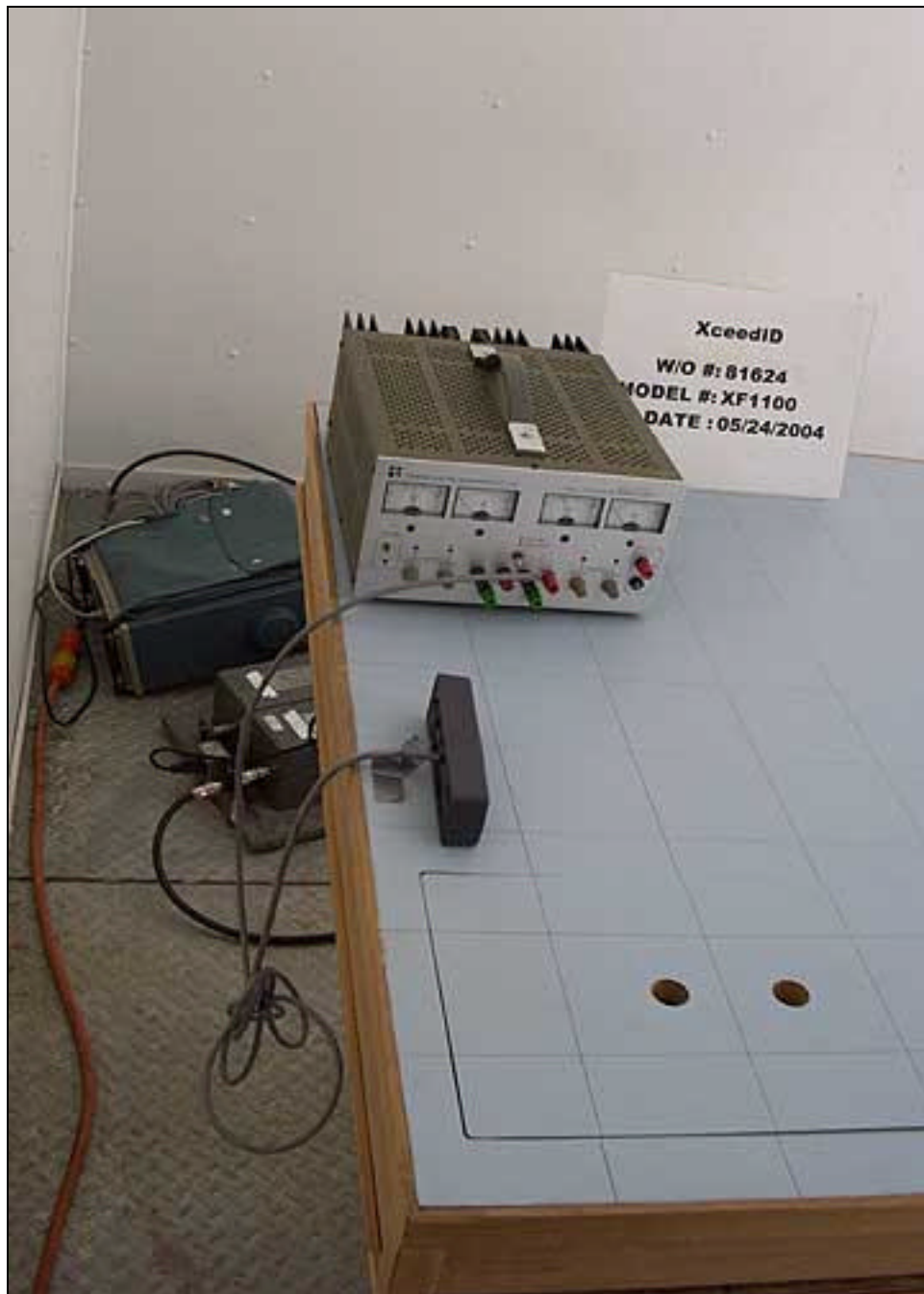
Mains Conducted Emissions - Side View
