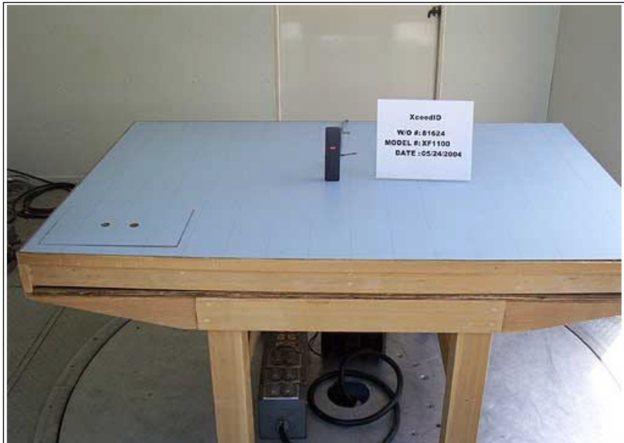
Radiated Emissions - Front View
