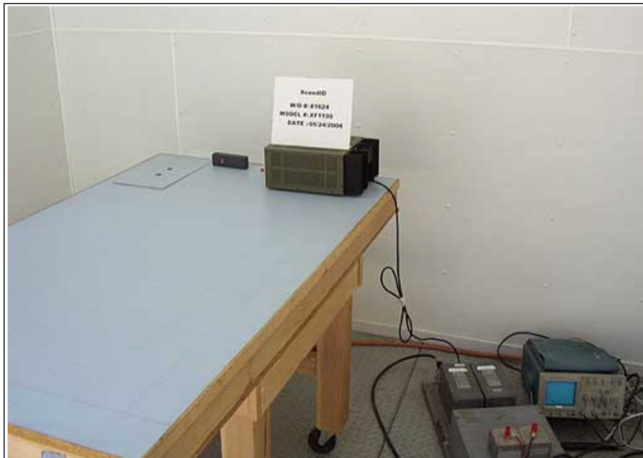
Mains Conducted Emissions - Front View
