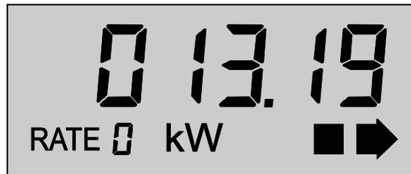
Figure 3-5. LCD displaying a sample 5-digit energy value for TOU rate C
