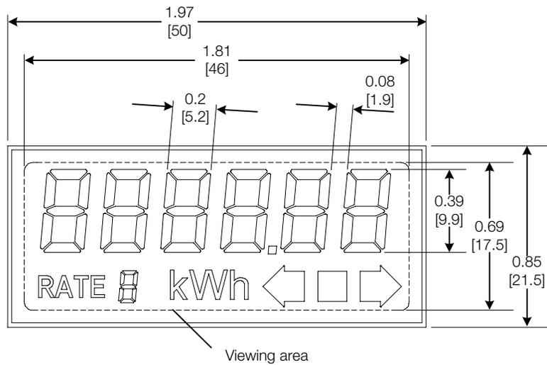
As shown in Figure 3-2, the LCD is divided into different display regions.
