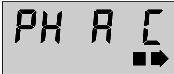
Figure B-9. Phase C voltage is not present (phase C < 50 V)
