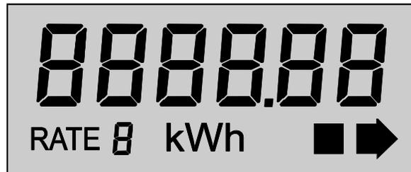
*Note: After power restoration, the LCD test always displays all segments (including the real energy arrows and square indicator) even if the LCD test is not selected as a displayable item.*
