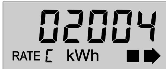
In addition, the REX meter can display the total energy value (see Figure B-5).
