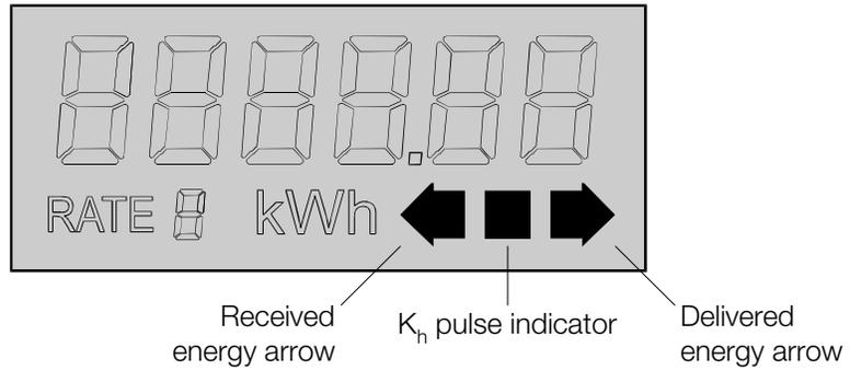
**Power/Energy Unit Identifier.** The power/energy unit identifier is used to indicate that the number displayed on the meter's LCD is either a demand or an energy value. When the value in the display quantity is a demand quantity, kW is displayed on the LCD, as shown in Figure 3-4. When the value in the display quantity is an energy quantity, kWh is displayed on the LCD, as shown in Figure 3-5.
