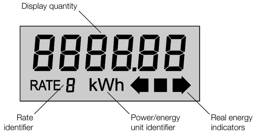
**Display Quantity.** This 6-digit display quantity on the LCD shows either metered quantities or other displayable information, depending upon how the REX meter was programmed either at the factory or using MAS. See Appendix B, “Display,” for more information.
