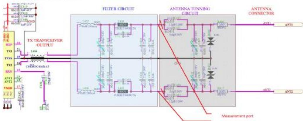
For this case Antenna Tuning Circuit was removed and antenna was disconnected
