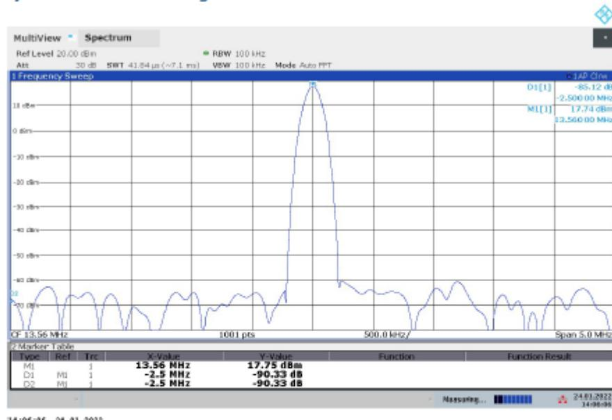
Result with matching circuit = 17,74 dBm = 59,42mW
