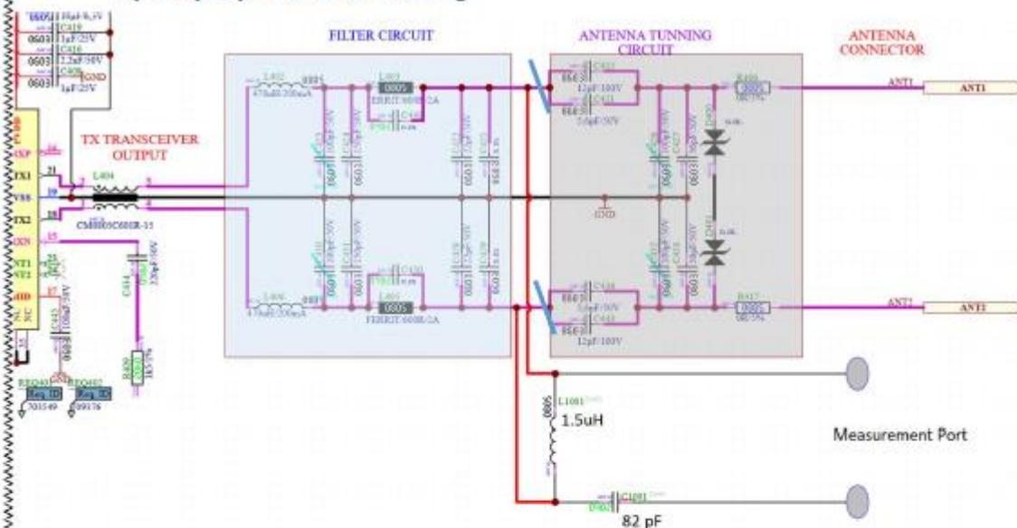
For this case Antenna Tuning Circuit was removed and antenna was disconnected, additional TX transceiver and Filter circuit was matched to 50 Ohm
