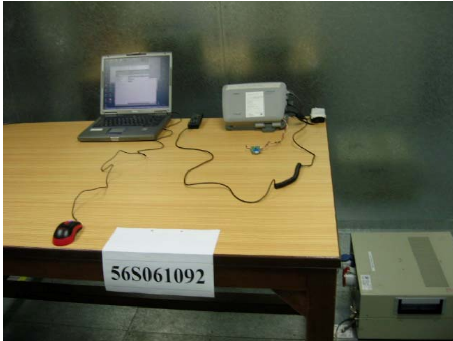
Conducted Emissions Test Setup (Front View)
