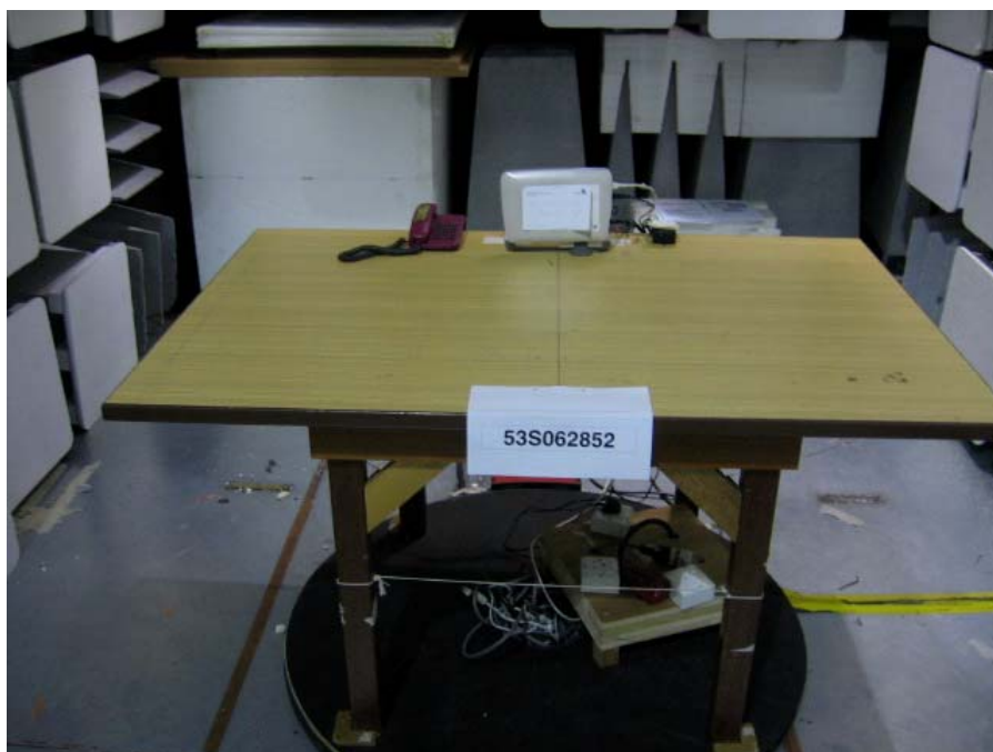
Band Edge Compliance (Radiated) Test Setup
