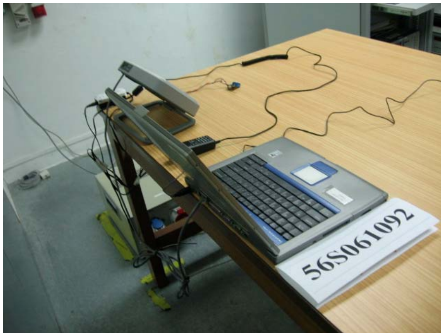
Conducted Emissions Test Setup (Rear View)
