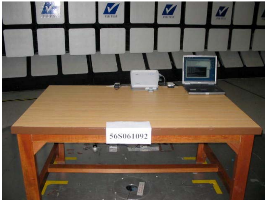
Radiated Emissions Test Setup (Front View)
