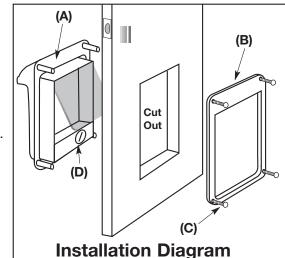
5. OPERATION - Place the round E-Z Pass Sensor on you pets collar. Insert the Power Cord in a household outlet and the Power Jack Plug into the DC Power Jack Receiver. Using the FUNCTION SWITCH (D) located on door's lower side, adjust to match the desired operation as indicated by embossed symbols on door (see Operation Diagram).
