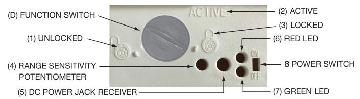
The Function switch has 3 positions, Unlocked (1), Active (2), and Locked (3). The Locked and Unlocked positions will override the function of the E-Z Pass receiver even if the Power Switch (8) is On. Only in the Active position (2) is the E-Z Pass receiver in control of the door if the Power Switch (8) in the On position and power is available.
