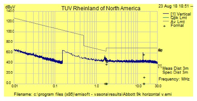
9k to 30MHz Horizontal unit in vertical orientation
