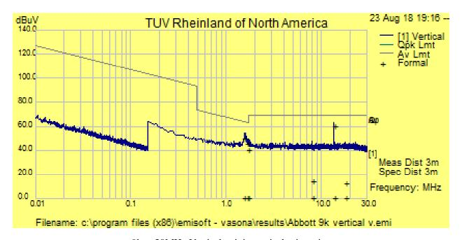
9k to 30MHz Vertical unit in vertical orientation
