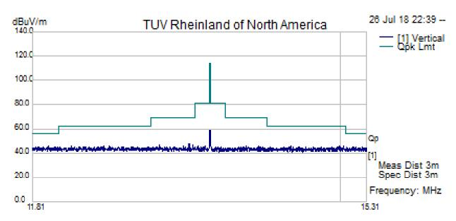
Filename: c:\program files (x88)\emisoft - vasona\results\donn\tgher.emi NFC mask requirement Horizontal unit in horizontal orientation
