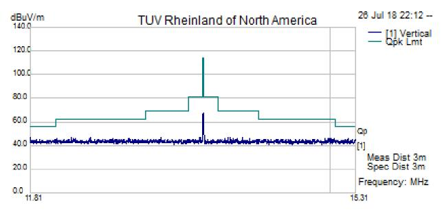
Filename: c:\program files (x88)\emisoft - vasona\results\donn\fhf.emi NFC mask requirement Vertical unit in vertical orientation
