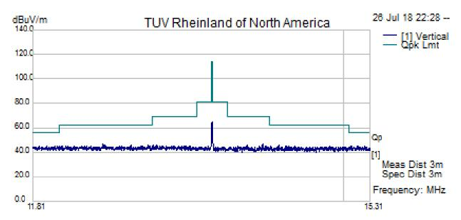
Filename: c:\program files (x88)\emisoft - vasona\results\donn\cchf.emi NFC mask requirement Vertical unit in horizontal orientation
