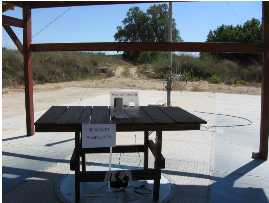
Figure 3. Radiated Emission Test Front
