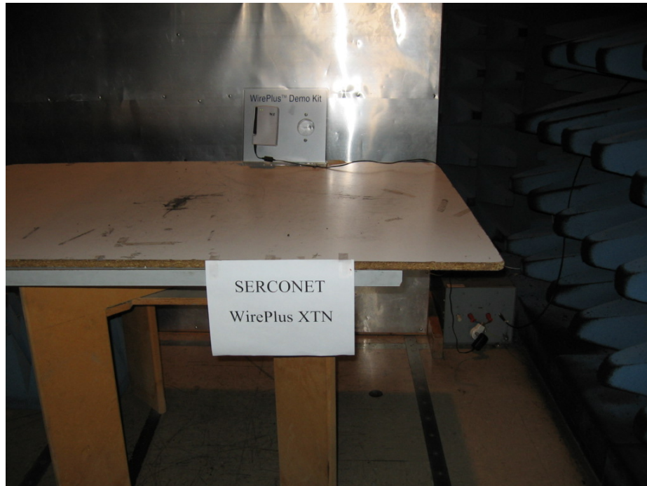
Figure 1. Conducted Emission From AC Mains Test Front
