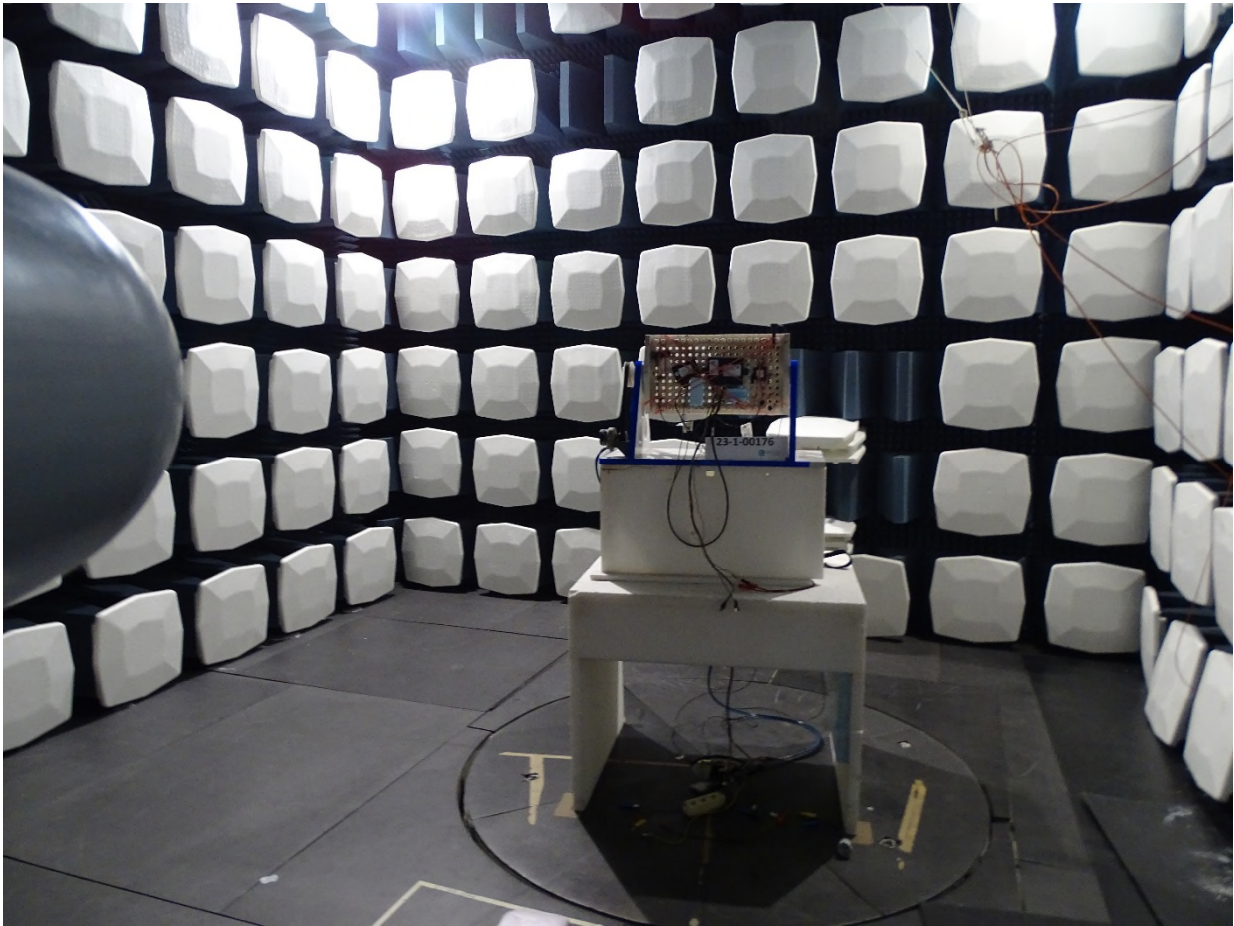
Fig. Mea.: 6 : Radiated RF Parameter external antenna Image 5
