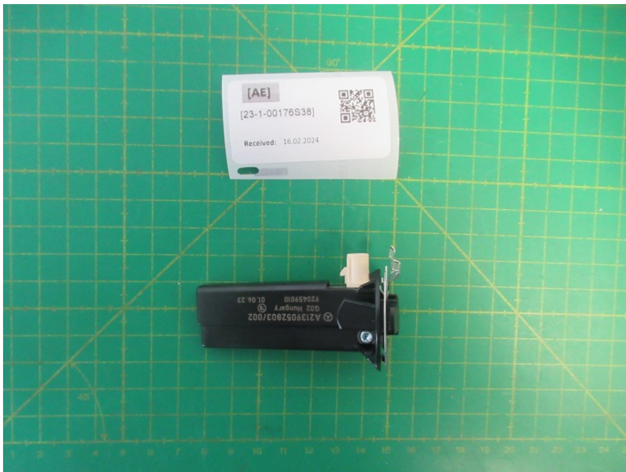
Fig. Ext.: 8 : Ext. - Front external cellular antenna
