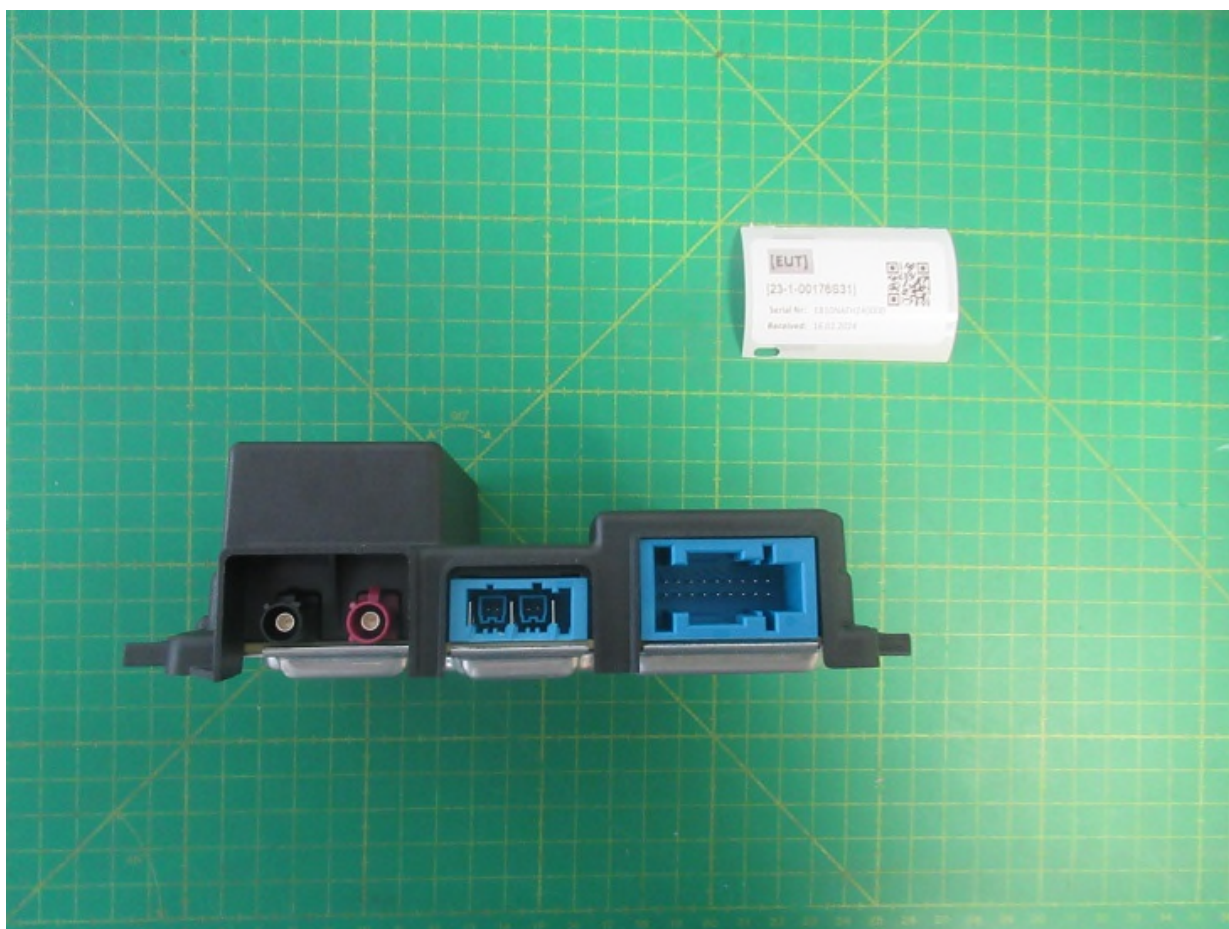
Fig. Ext.: 2 : Ext. - Special Emergency call control unit
