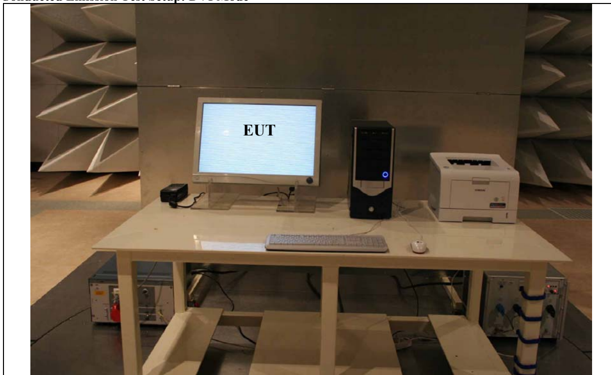
Figure 1 Conducted Emission Test Setup: DVI Mode
