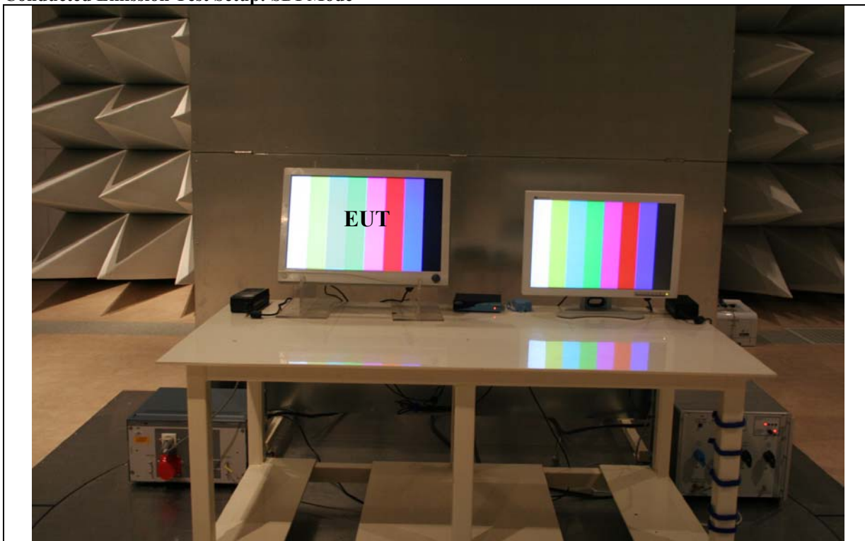
Figure 2 Conducted Emission Test Setup: SDI Mode
