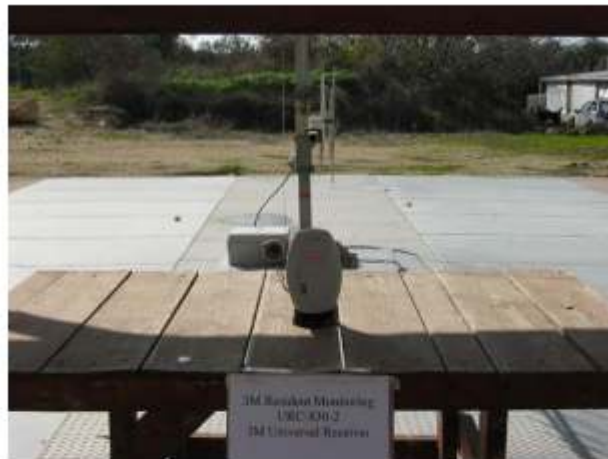
Figure 4. Radiated Emission Test 30 MHz – 1 GHz
