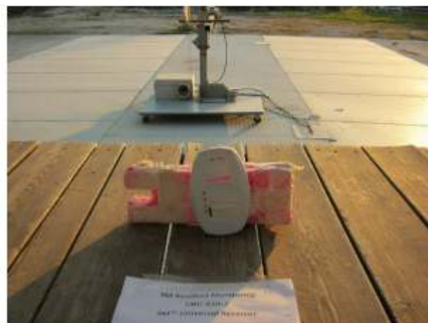
Figure 5. Radiated Emission Test 1 GHz - 4.5 GHz
