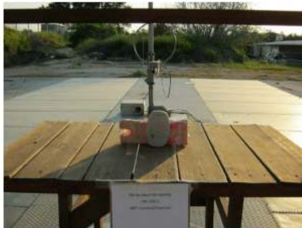
Figure 3. Radiated Emission Test 9 KHz - 30 MHz
