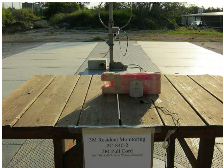
Figure 3. Radiated Emission Test 9KHz-30MHz
