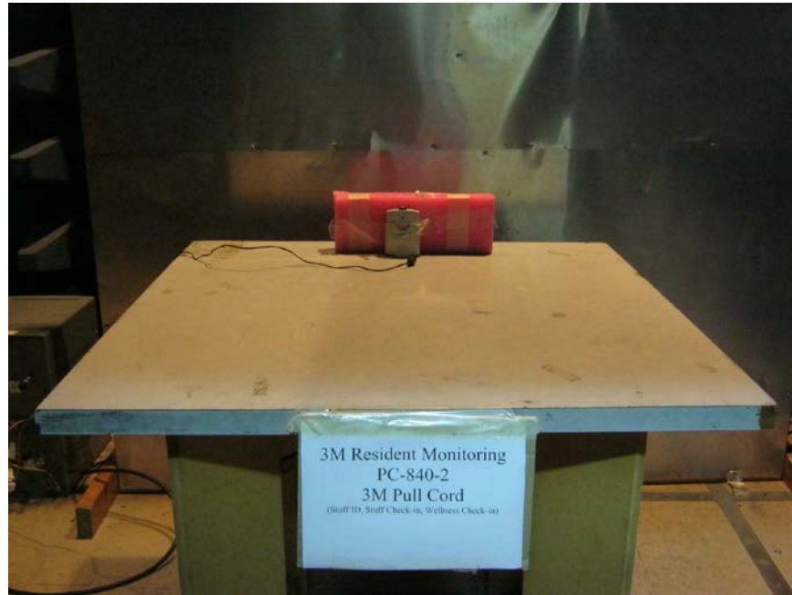
Figure 2. Conducted Emission Test
