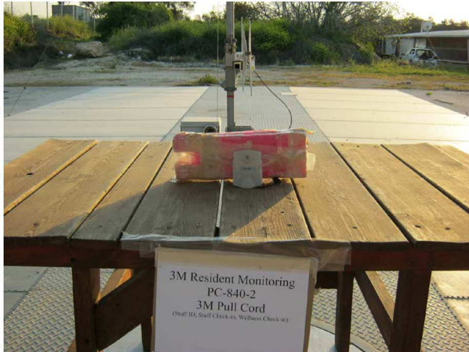
Figure 4. Radiated Emission Test 30 MHz-4500MHz
