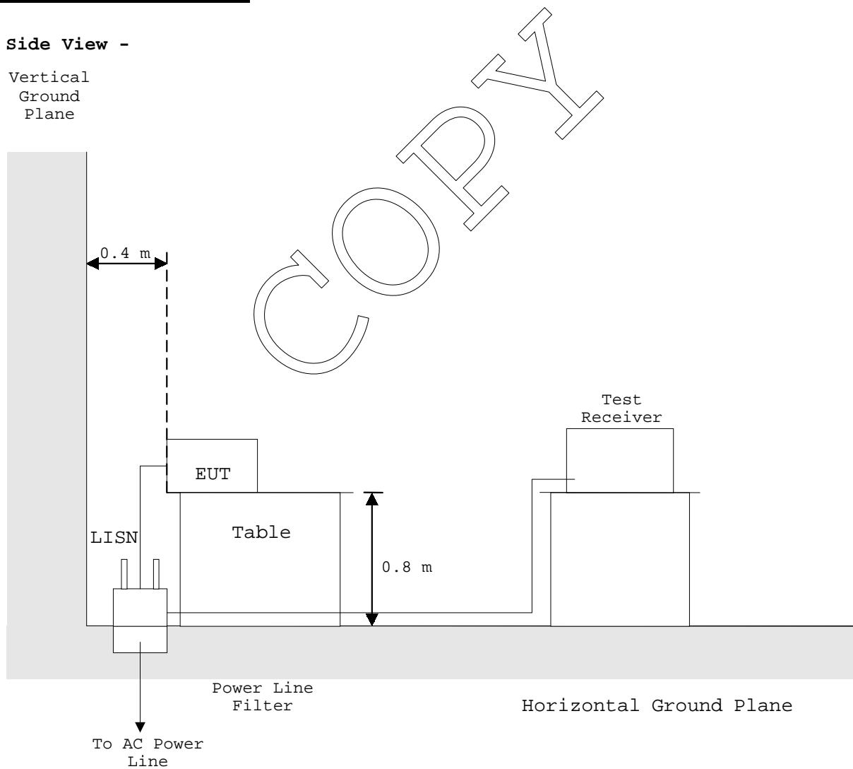
**1.9.2 Radiated Emission ( 9 kHz - 30 MHz) :**
