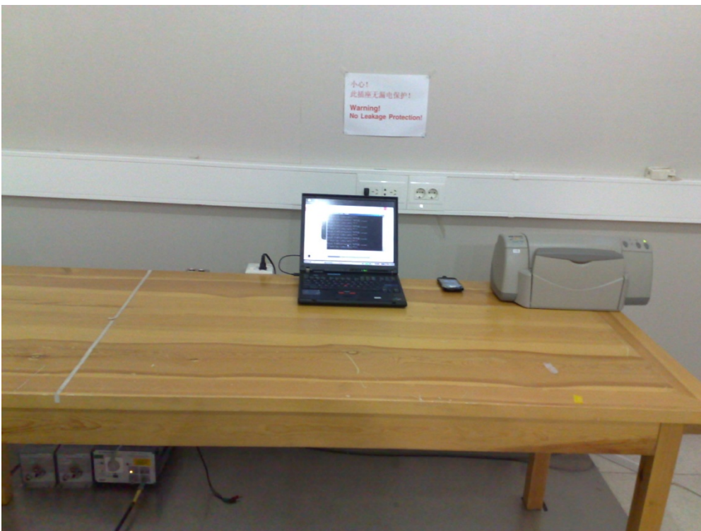
Picture 5. FCC Part 15B AC powerline conducted emissions, computer peripherals
