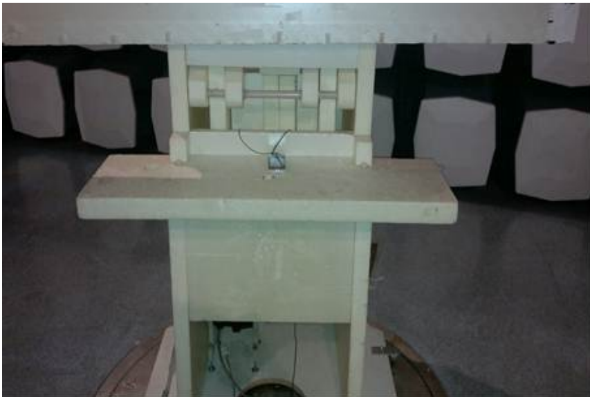
Picture 2. FCC Part 15B Radiated emissions
