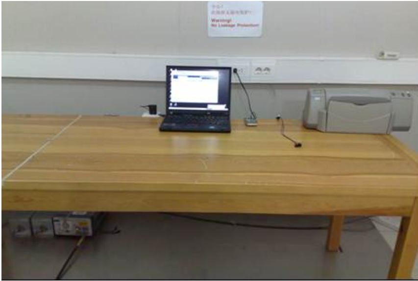
Picture 5. FCC Part 15B AC powerline conducted emissions, computer peripherals, measure from phone charger
