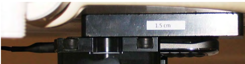
Photo of the device positioned for Body SAR measurement. The spacer was removed for the tests.
