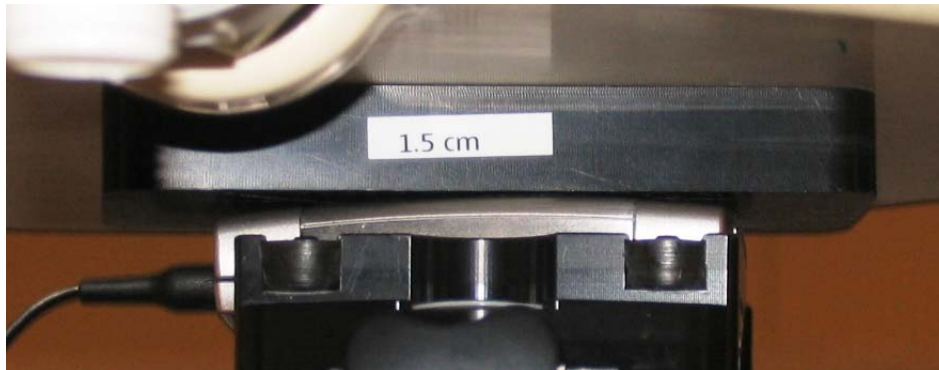
Photo of the device positioned for Body SAR measurement. The spacer was removed for the tests.
