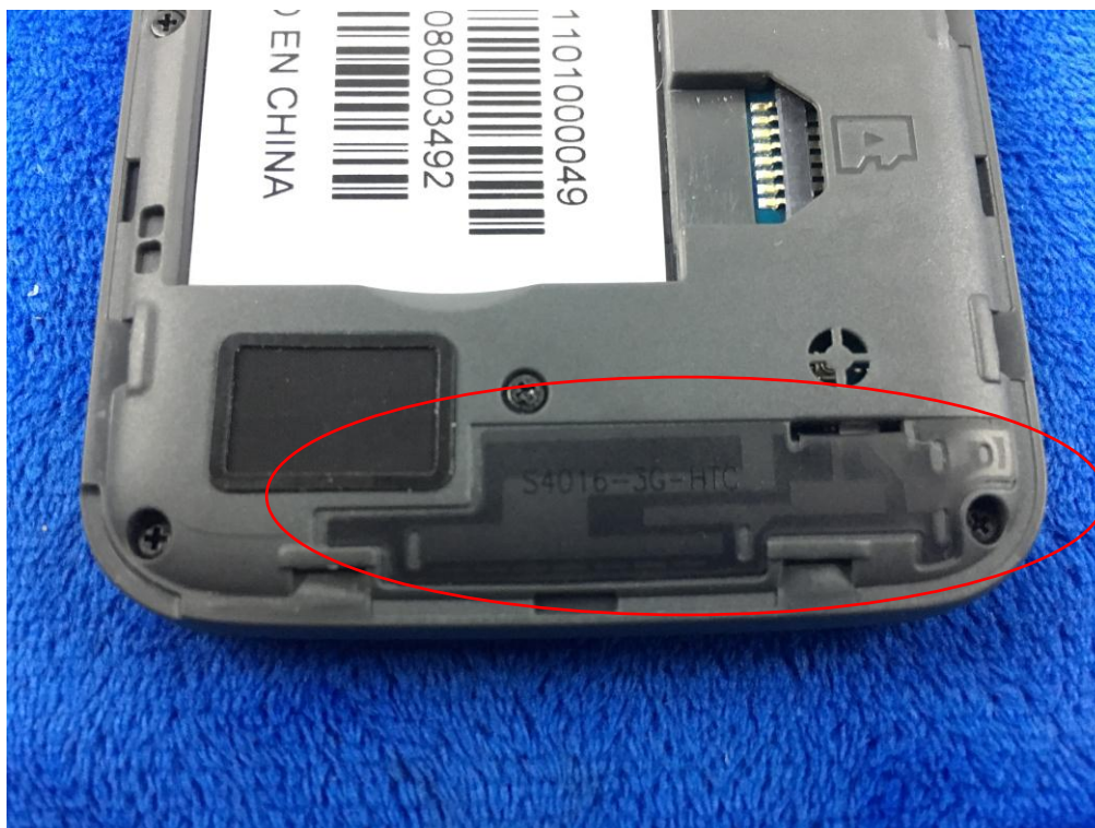
GSM/PCS/UMTS-FDD Antenna View
