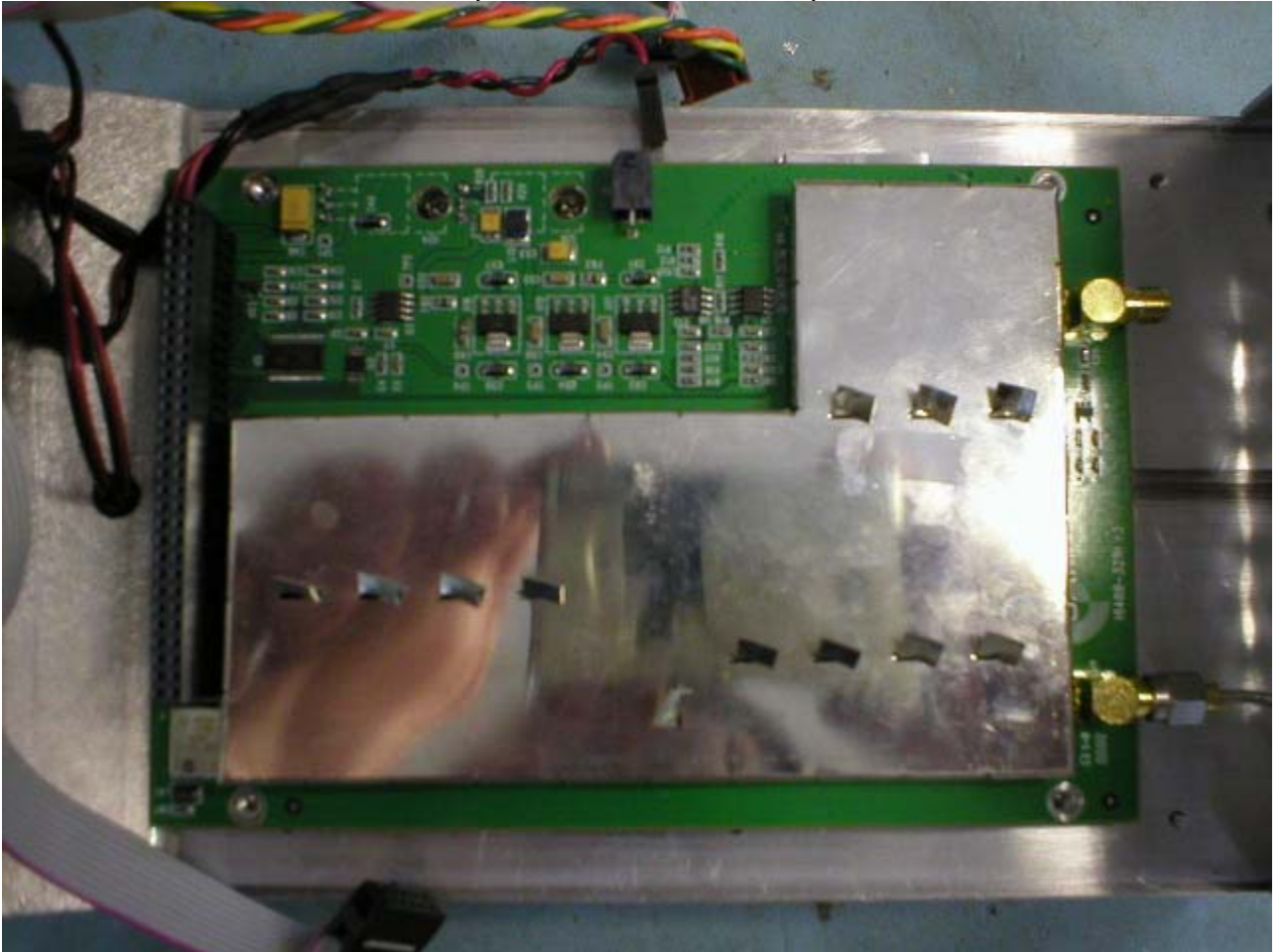
Board 4 – Component Side – Shield in place
