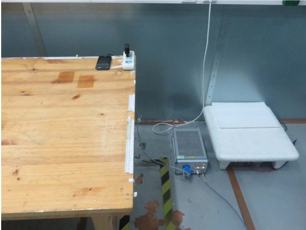
Picture 3 Conducted Emission Test Setup
