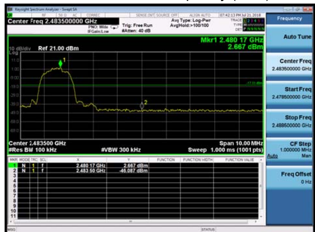
BT 3DH5 CH78, Carrier frequency (MHz):2480
