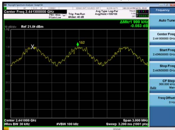
BT DH5 CH78, Carrier frequency (MHz):2480
