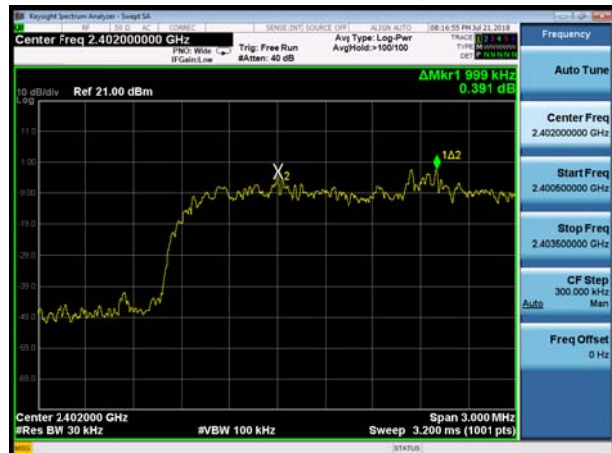
BT 2DH5 CH39, Carrier frequency (MHz): 2441
