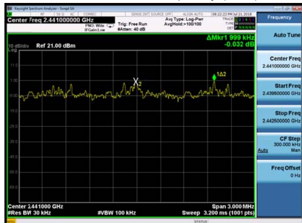
BT 2DH5 CH78, Carrier frequency (MHz):2480
