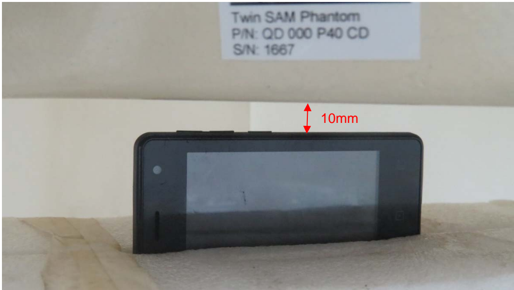
Right Side, the distance from handset to the bottom of the Phantom is 10mm
