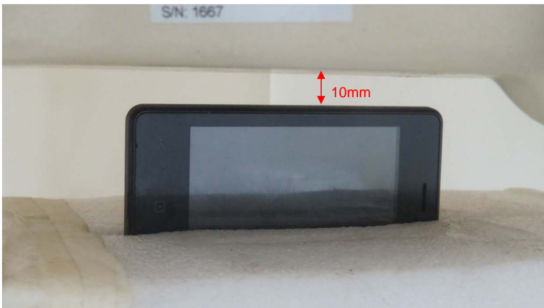
Left Side, the distance from handset to the bottom of the Phantom is 10mm
