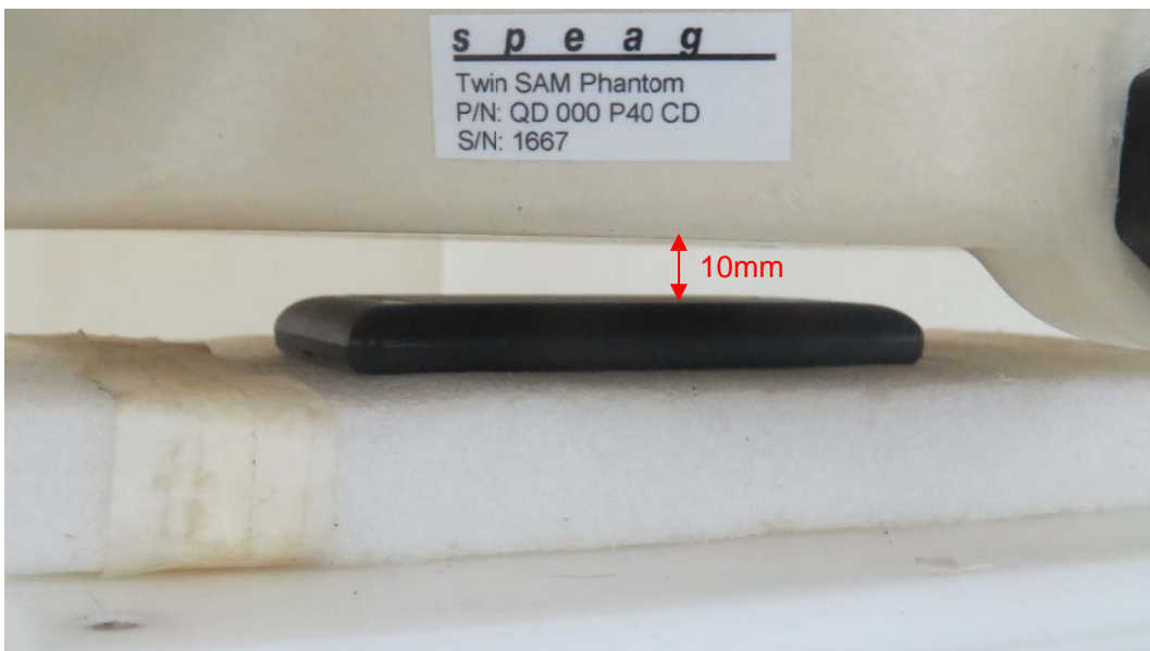
Back Side, the distance from handset to the bottom of the Phantom is 10mm
