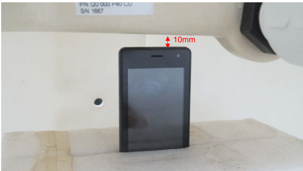
Top Side, the distance from handset to the bottom of the Phantom is 10mm
