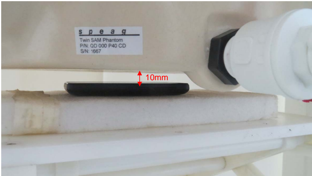
Front Side, the distance from handset to the bottom of the Phantom is 10mm
