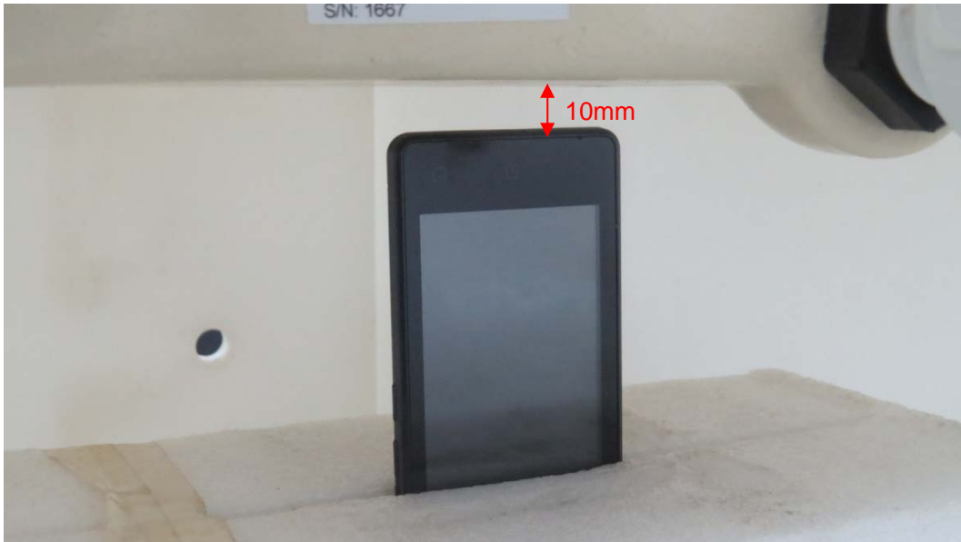
Bottom Side, the distance from handset to the bottom of the Phantom is 10mm
