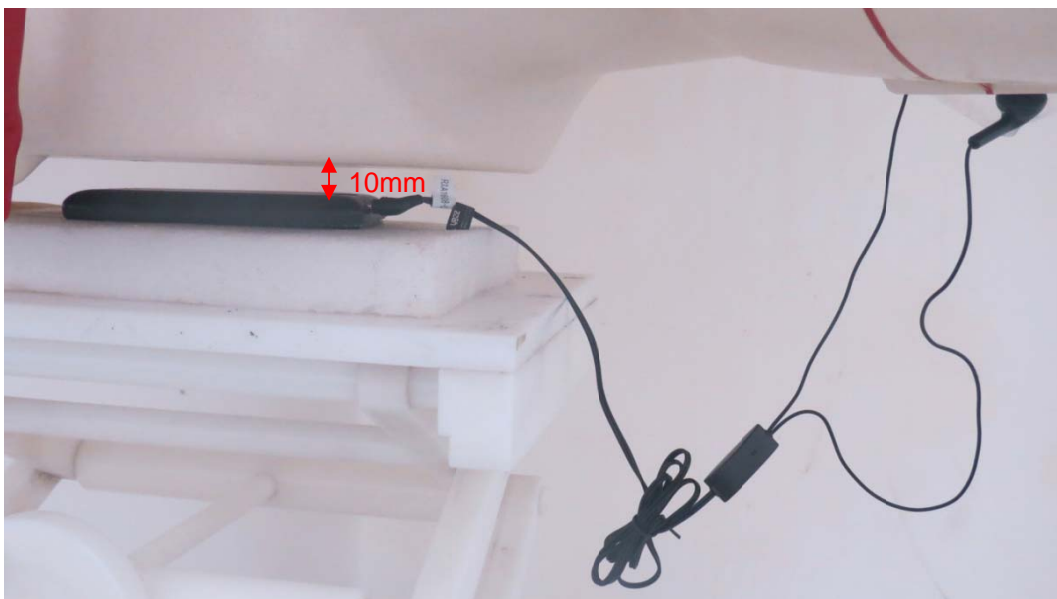
Back Side with Earphone, the distance from handset to the bottom of the Phantom is 10mm
