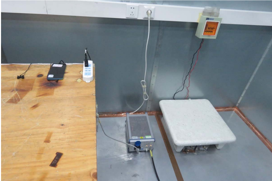
Picture 2 Conducted Emission Test Setup
