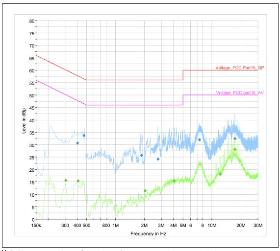
Note:Blue trace uses the peak detection Green trace uses the average detection
