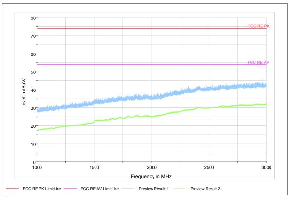
Note:Blue trace uses the peak detection Green trace uses the average detection
