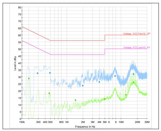
Note:Blue trace uses the peak detection Green trace uses the average detection N line
