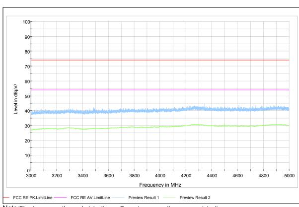
Note:Blue trace uses the peak detection Green trace uses the average detection
