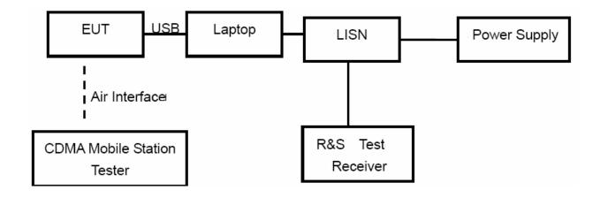
Note: Power Supply is AC Power source and it is used to change the voltage from 220V/50Hz to 110V/60Hz.
