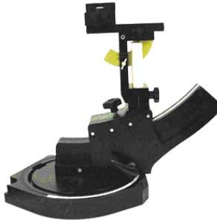
Device holder supplied by SPEAG
