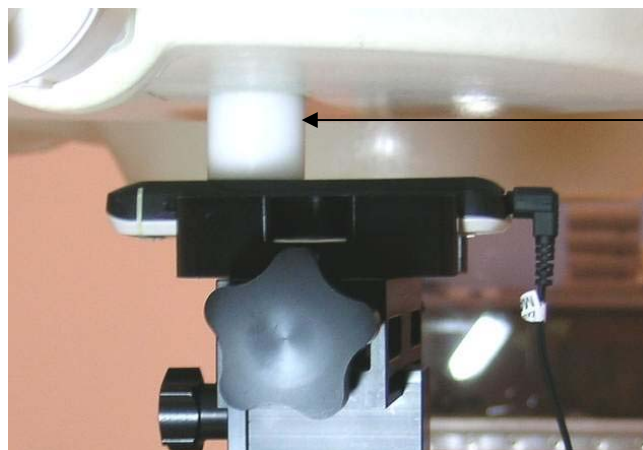
Photo of the device positioned for Body SAR measurement. The spacer was removed for the tests.
