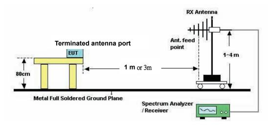
For conducted emissions above 960MHz (Conducted antenna port measurement)
