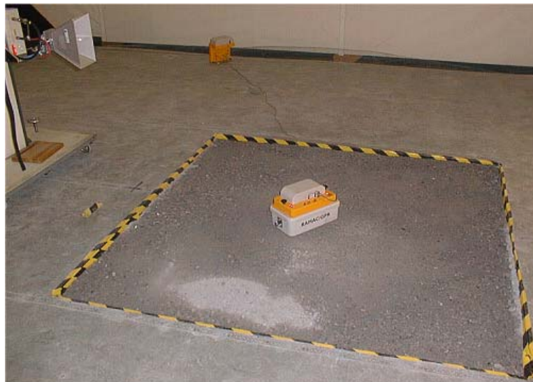
Picture 2: EUT set-up on sand bed
