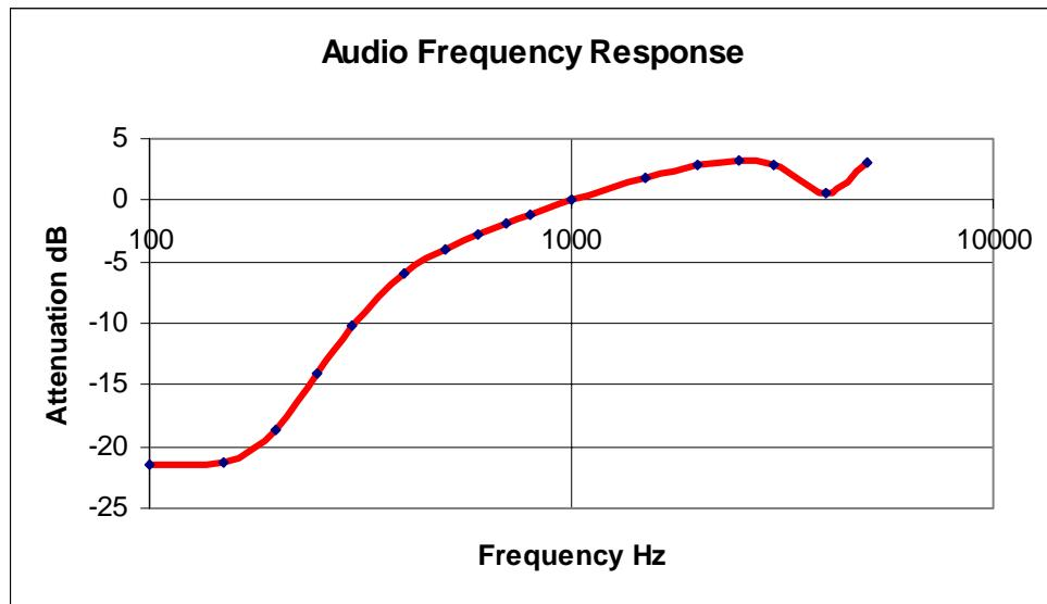
2.1047(b) Audio input versus modulation
