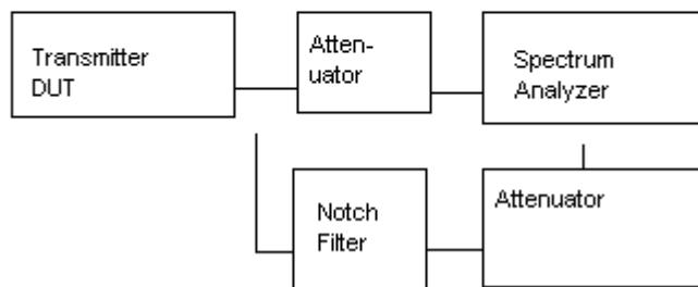
Method of Measuring Conducted Spurious Emissions
