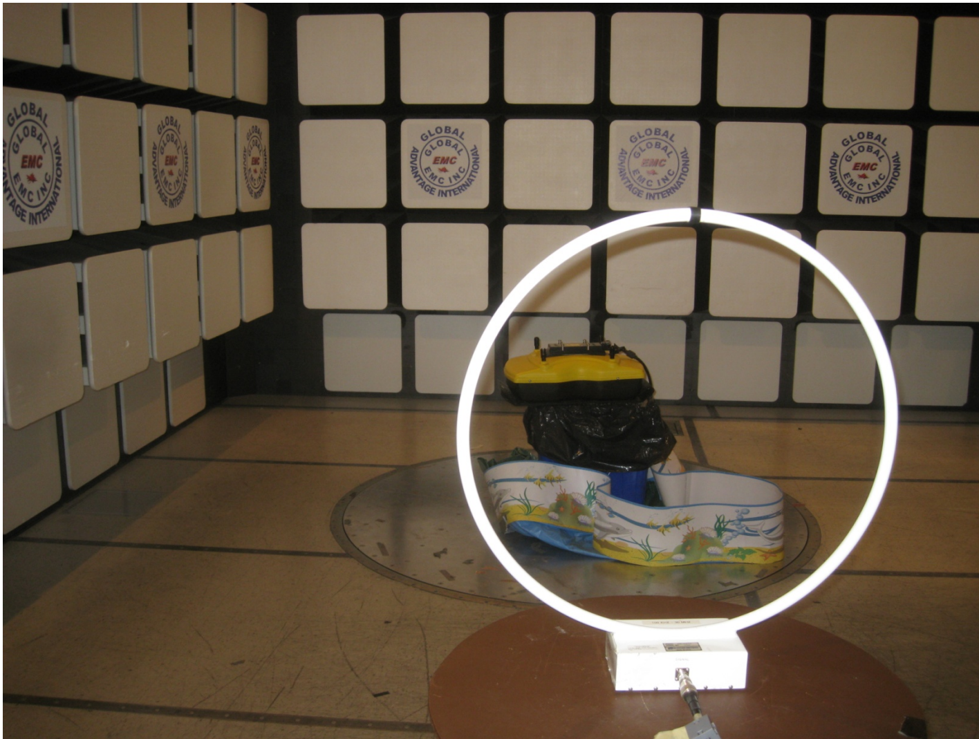
Radiated Emissions Setup (Below 30 MHz)
