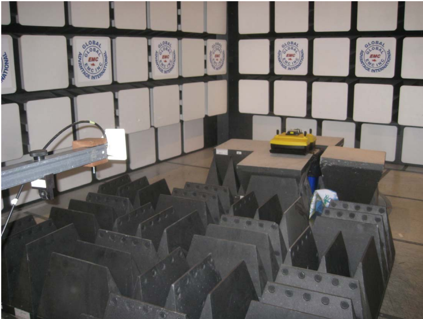
Radiated Emissions – High Frequency setup
