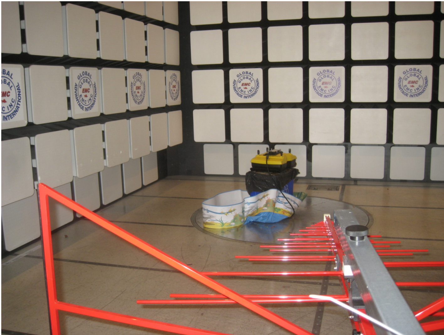
Radiated Emissions Setup (30 MHz to 960 MHz)
