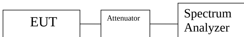
Figure 4. Power Spectral Density Test Setup
