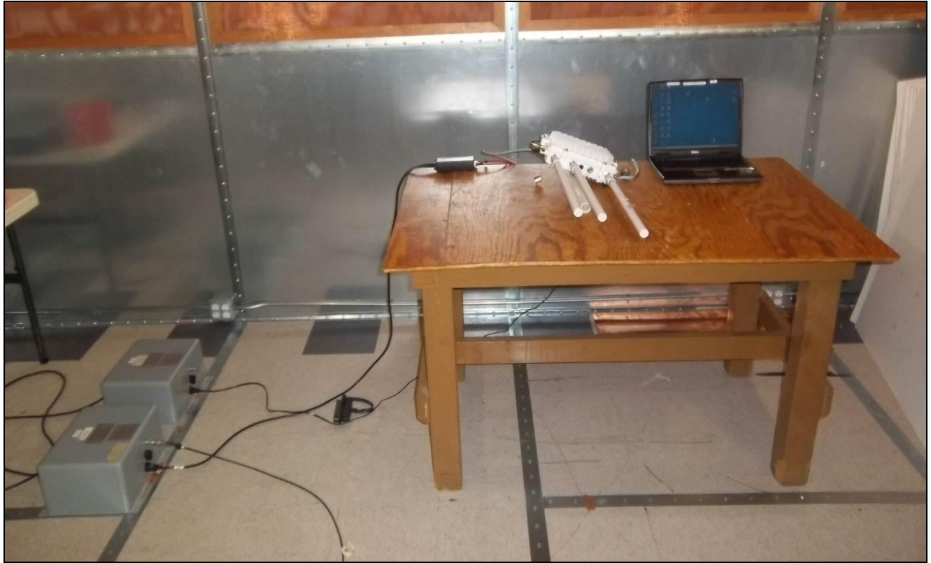
Photograph 2. Conducted Emissions, Test Setup
