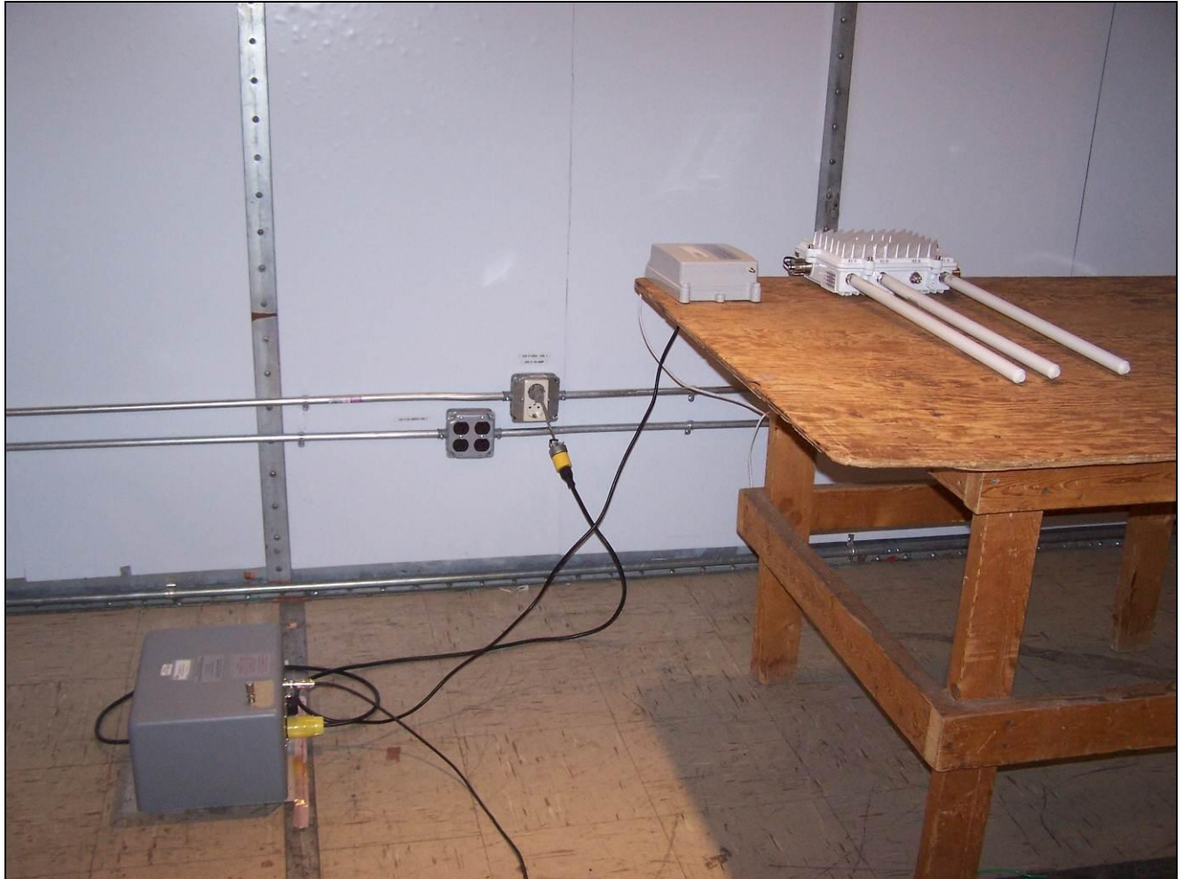
Photograph 4. Conducted Emissions, Test Setup
