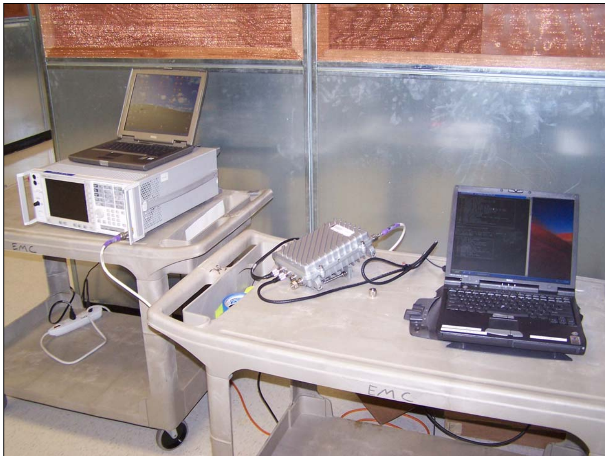
Photograph 7. Peak Power Spectral Density Test Setup
