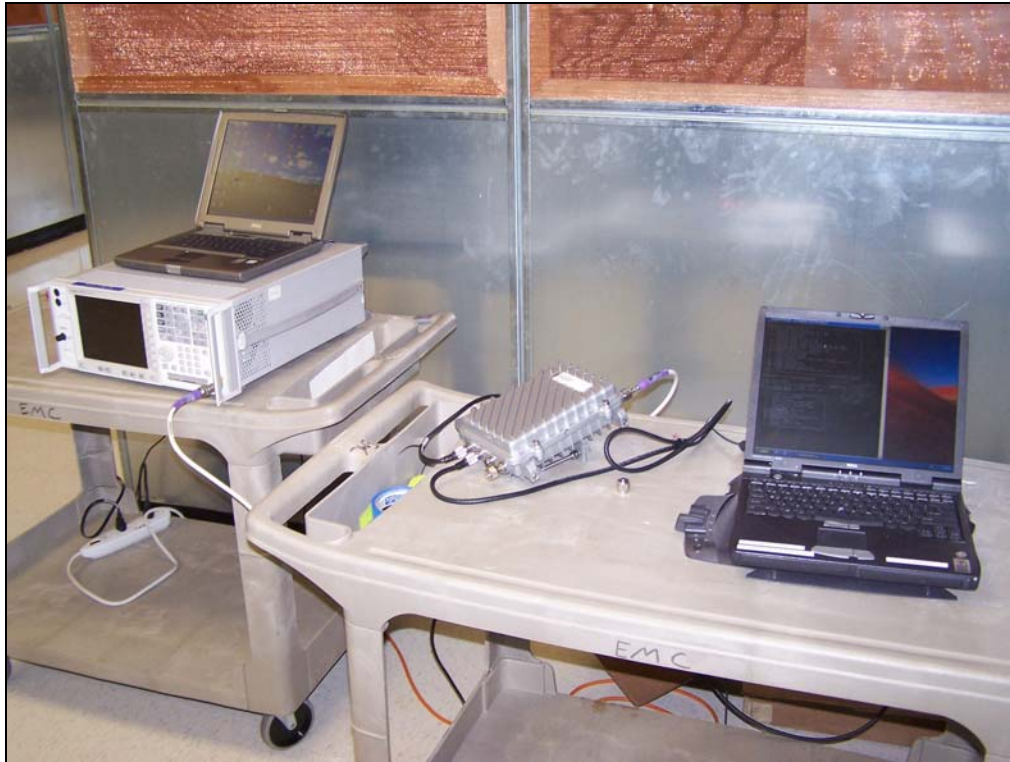
Photograph 5. Peak Power Output, Test Setup
