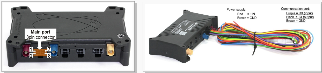
Figure 2: Pin assignments of 8-pin (2x4) connector and installation cable connection (CA39 with 2A fuse).
