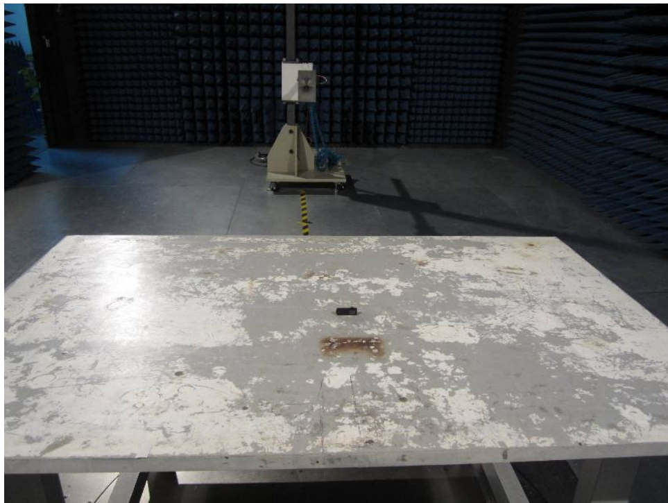
Setup for Radiated Emission
