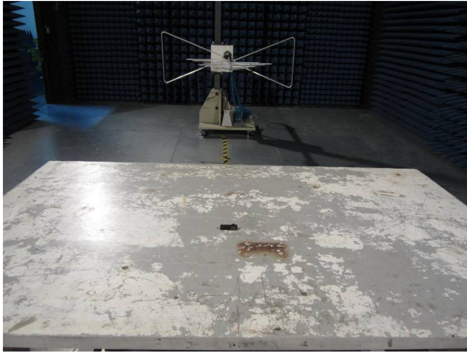
Setup for Radiated Emission
