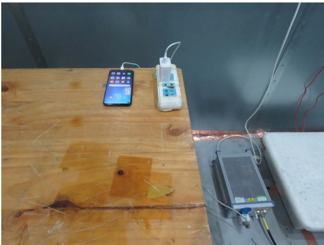
Picture 2 Conducted Emission Test Setup
