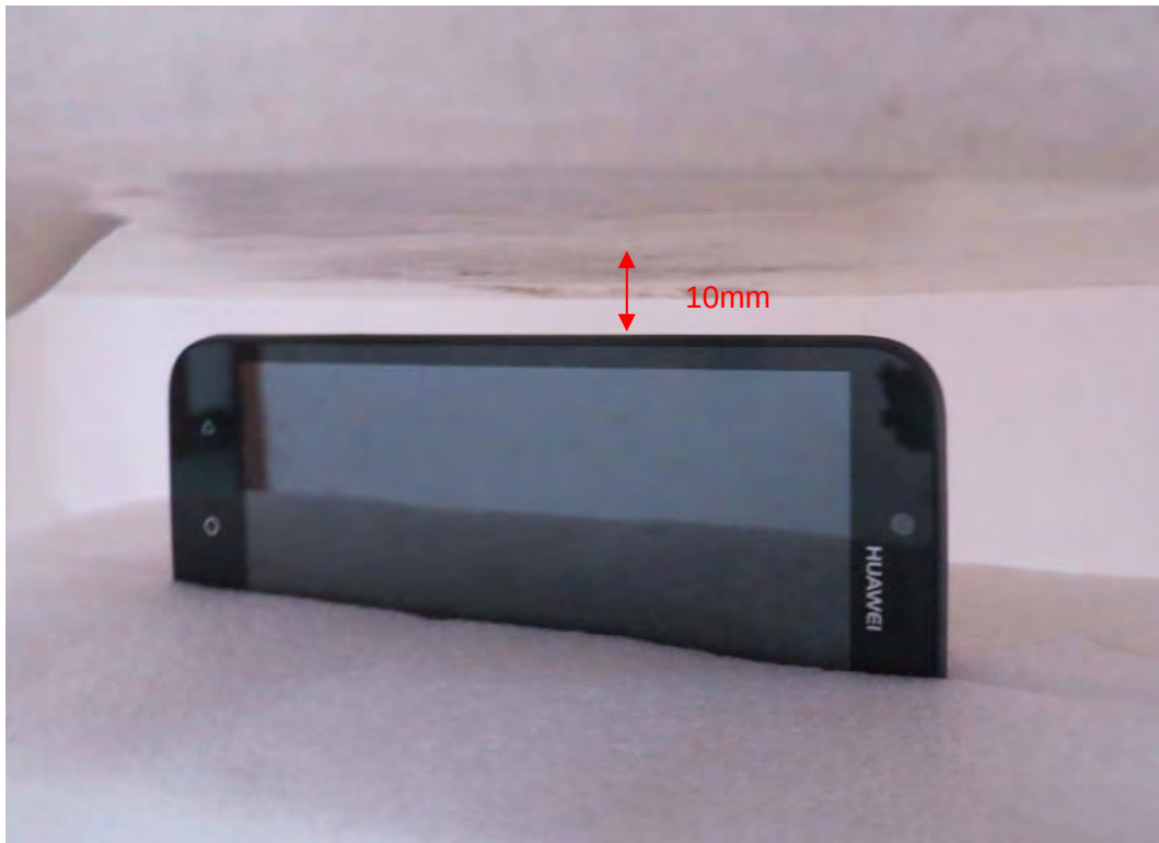
Picture 15: Left Edge, the distance from handset to the bottom of the Phantom is 10mm (Original Model)
