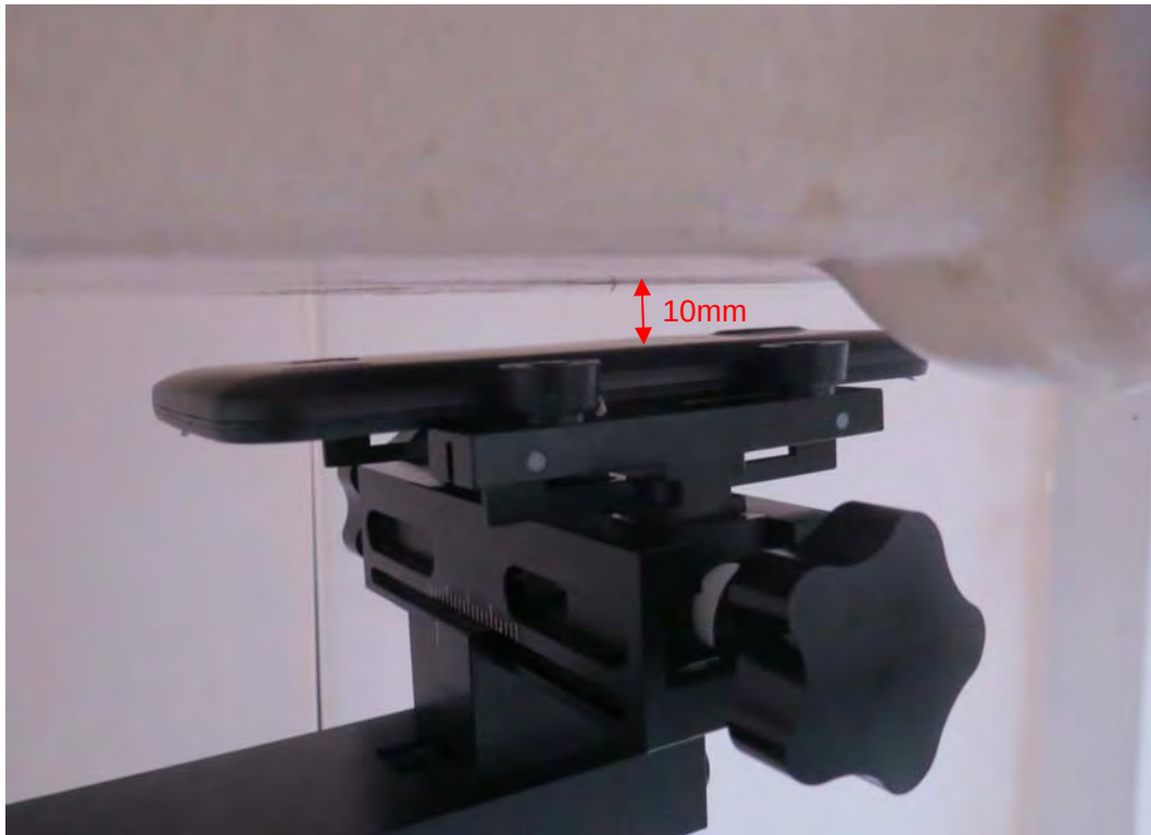
Picture 13: Back Side, the distance from handset to the bottom of the Phantom is 10mm (Original Model)
