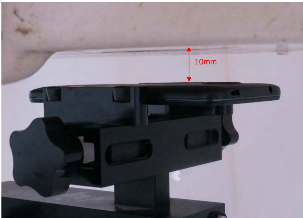
Picture 21: Back Side, the distance from handset to the bottom of the Phantom is 10mm (Variant Model)
