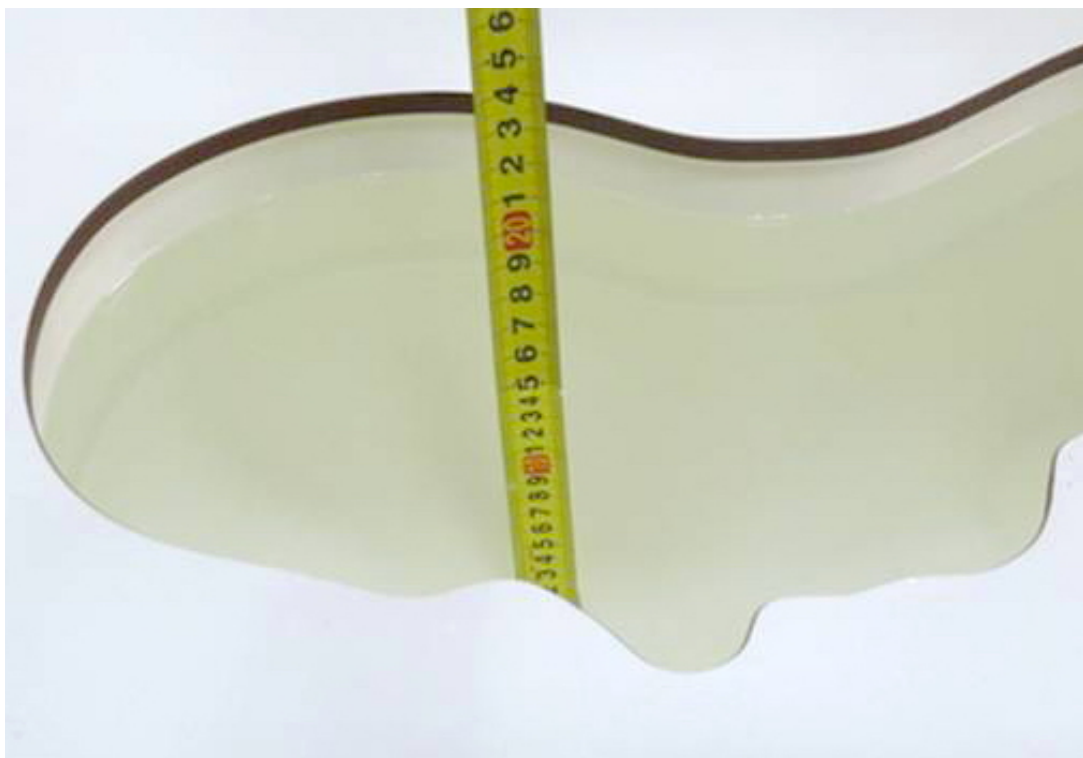
Picture : liquid depth in the head Phantom (1900 MHz, 15.3cm depth)
