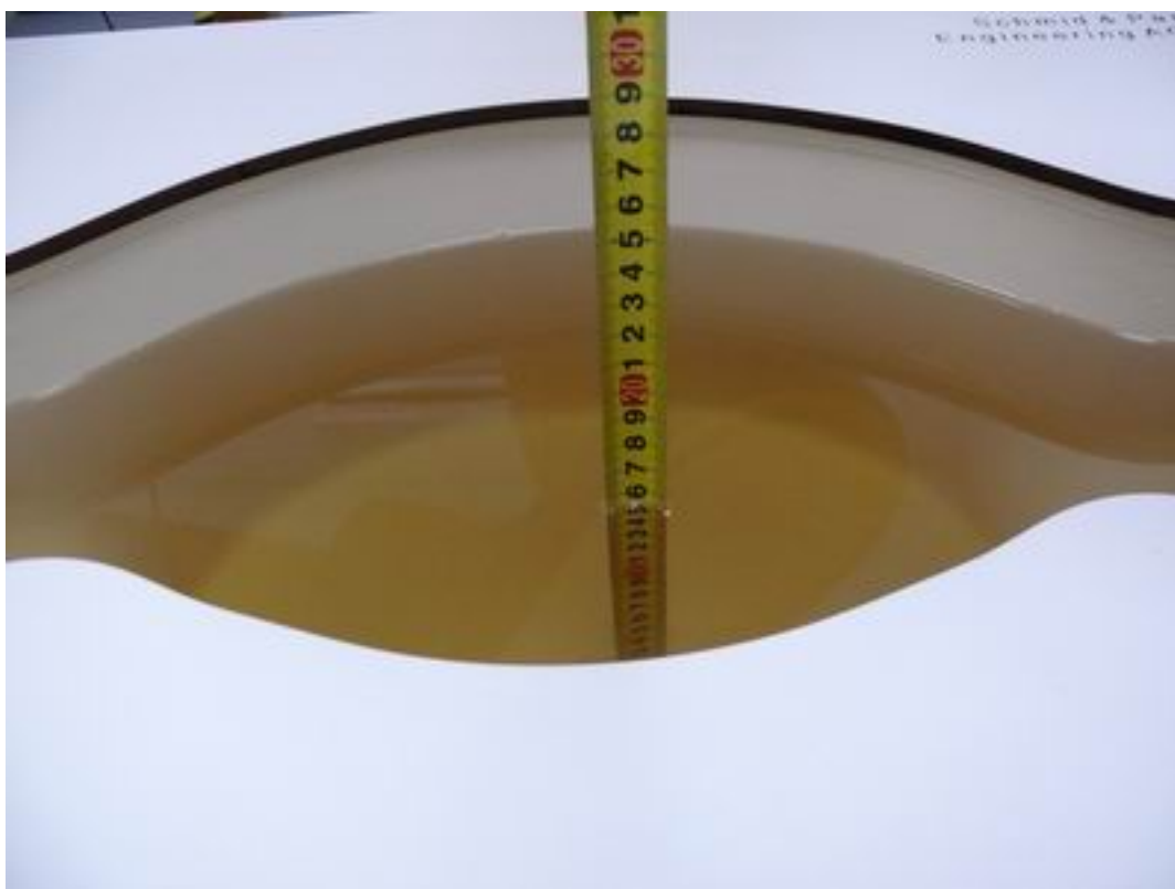
Picture : Liquid depth in the flat Phantom (835MHz, 15.4cm depth)
