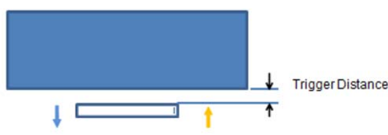
Picture: Proximity sensor triggering distances assessment Front Side and Back side
