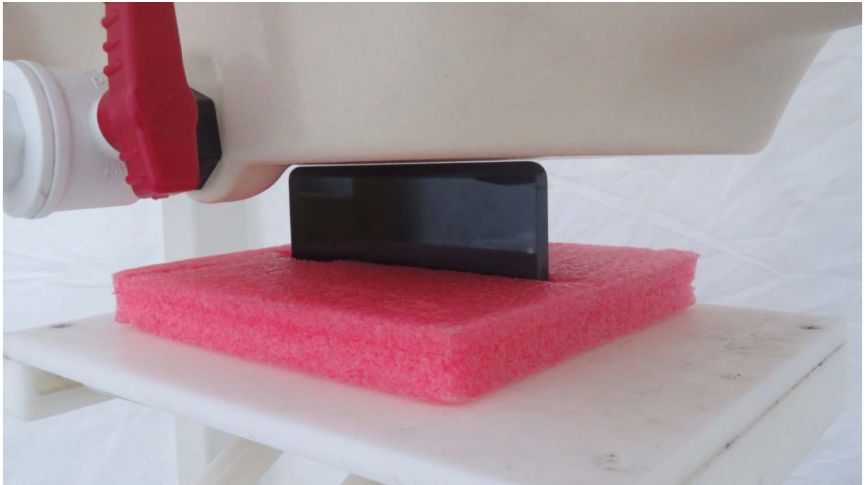
Picture 15: Left Side, the distance from handset to the bottom of the Phantom is 0mm
