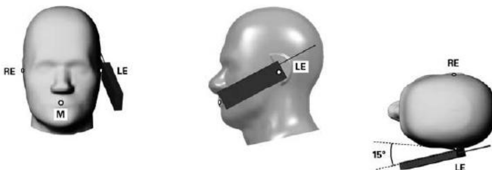
Figure 3 Front, Side and Top View of Tilt 15° Position
