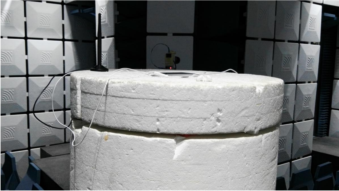
Radiated Spurious Emission (18GHz to26.5GHz)
