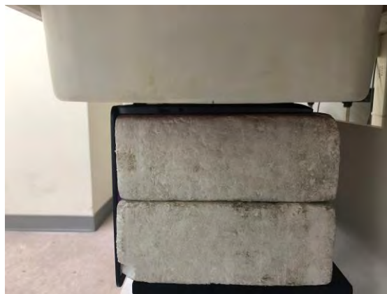
Fig.3 EUT Bottom side to flat phantom
