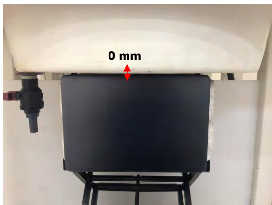
Fig.3 EUT Bottom side to flat phantom
