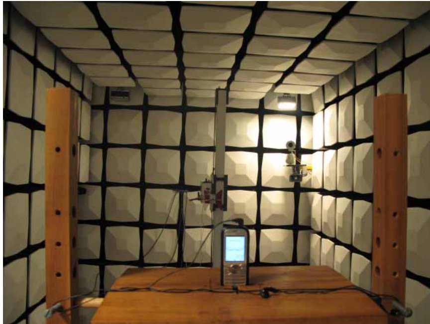
Radiated Spurious Emission (2GHz to18GHz)
