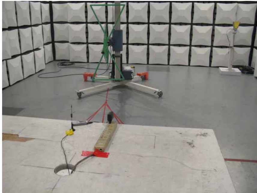
Radiated Spurious Emission (below 2GHz)
