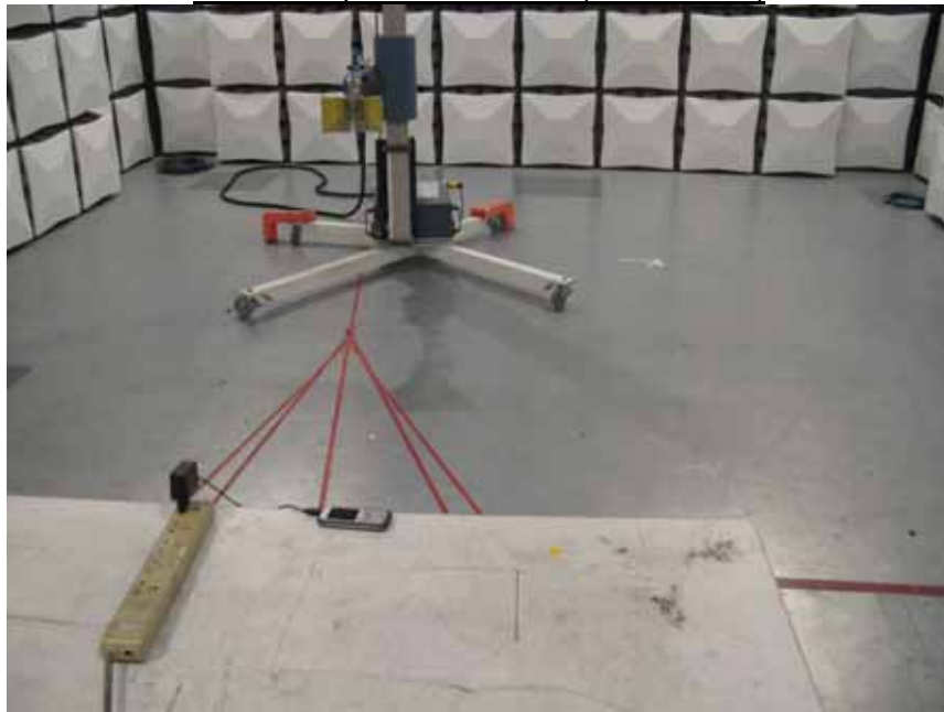
Radiated Spurious Emission (2GHz to 18GHz)
