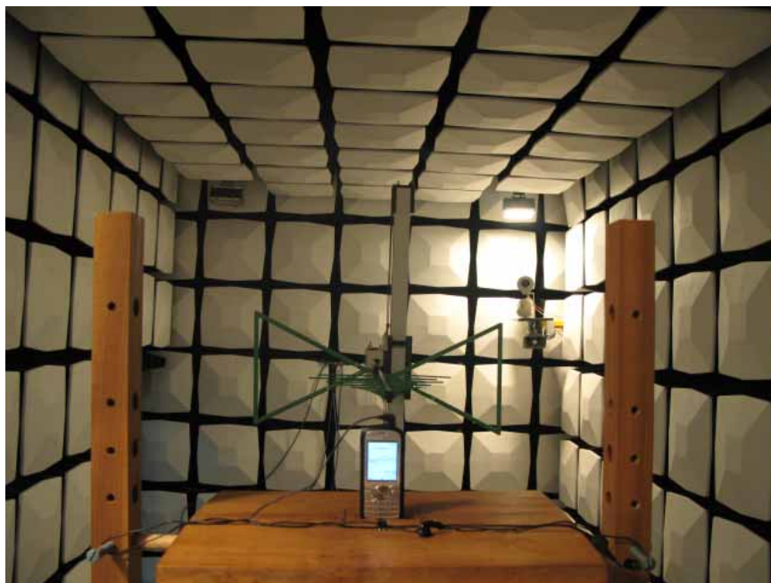
Radiated Spurious Emission (below 2GHz)
