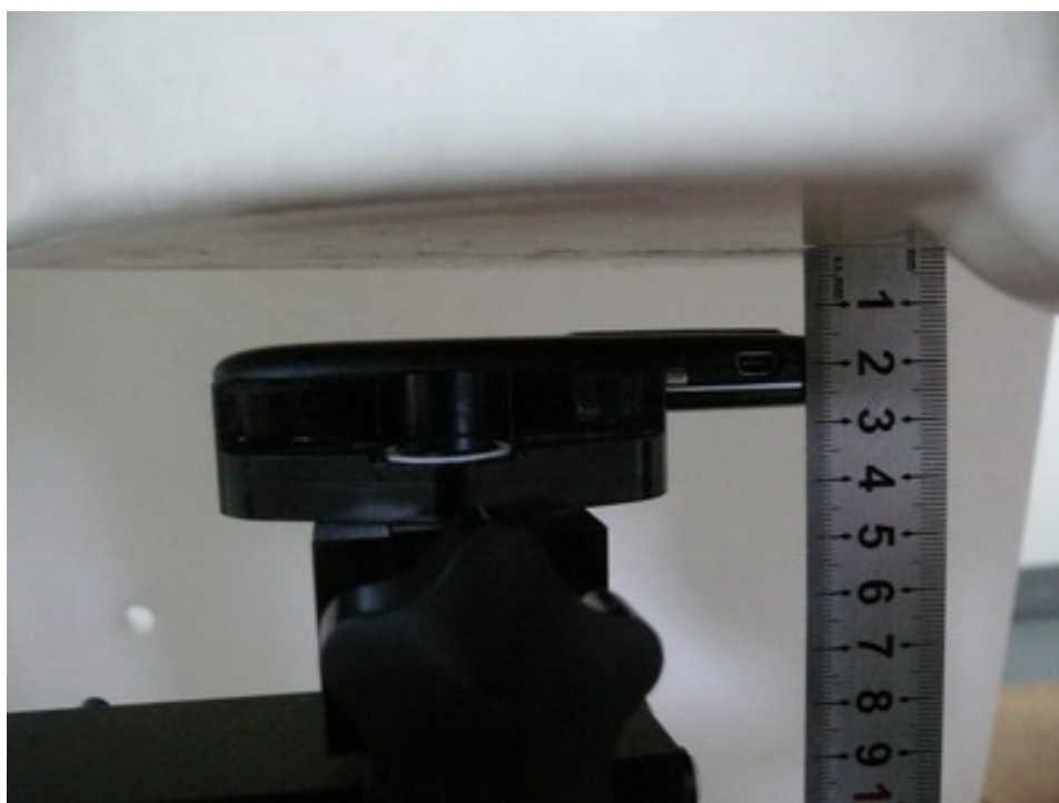
Picture 9: Body, The EUT display towards ground, the distance from handset to the bottom of the Phantom is 15mm
