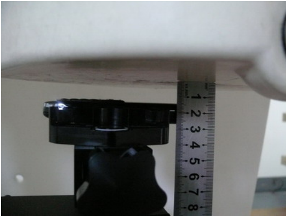
Picture 10: Body, The EUT display towards phantom, the distance from handset to the bottom of the Phantom is 15mm
