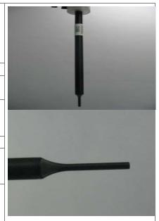
Isotropic E-Field Probe EX3DV4 for Dosimetric Measurements
