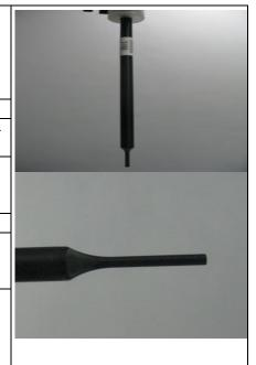
Isotropic E-Field Probe EX3DV4 for Dosimetric Measurements
