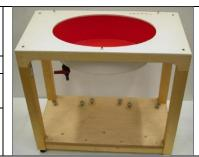
The ELI4 phantom is intended for compliance testing of handheld and body-mounted wireless devices in the frequency range of 30MHz to 6GHz. ELI4 is fully compatible with the latest draft of the standard IEC 62209-2 and all known tissue simulating liquids.
