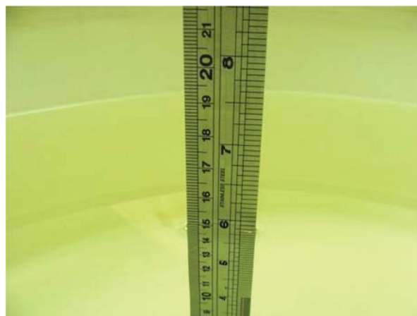
Fig 6.2 Photo of Liquid Height for Body SAR
