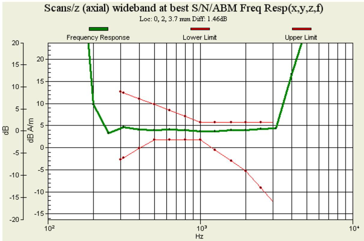
Figure 22 T-Coil WCDMA Band IV Z Axial
