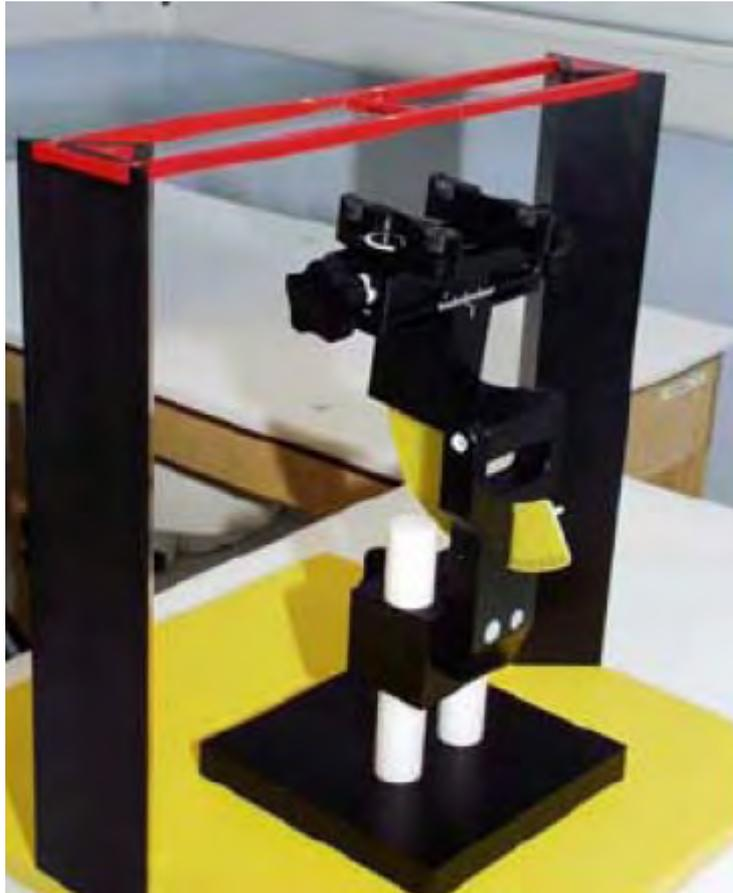
**Figure 7 T-coil Phantom & Device Holder**
