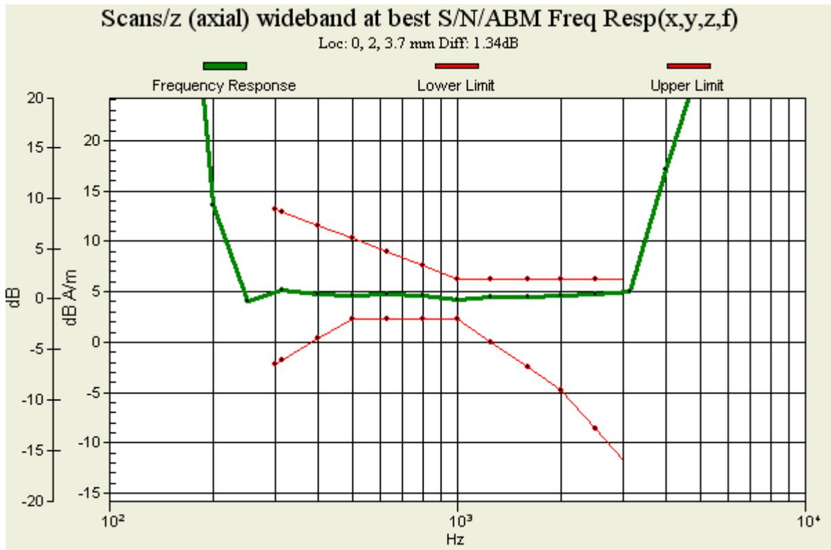
Figure 19 T-Coil WCDMA Band II Z Axial
