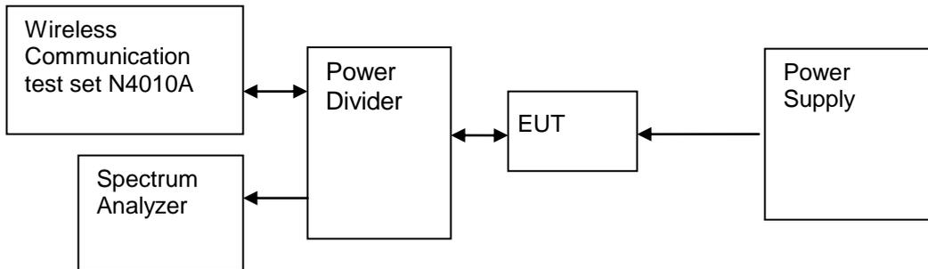
Figure 4. Test Set-up
