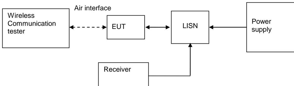
Figure 9. Test Set-up
