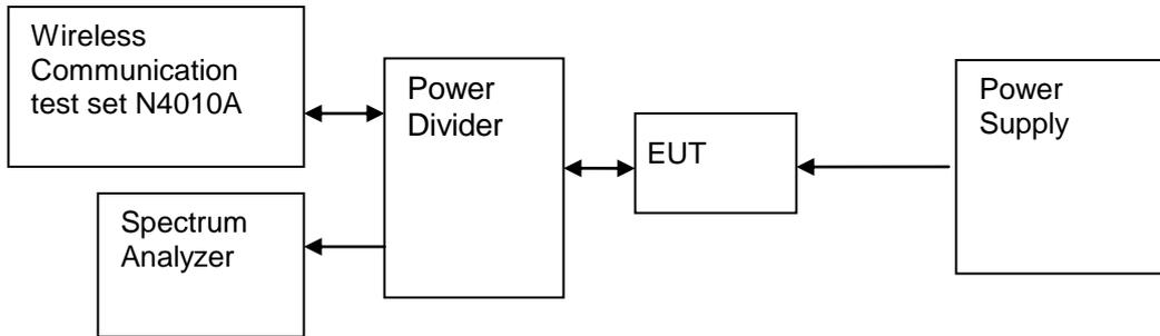
Figure 7. Test Set-up
