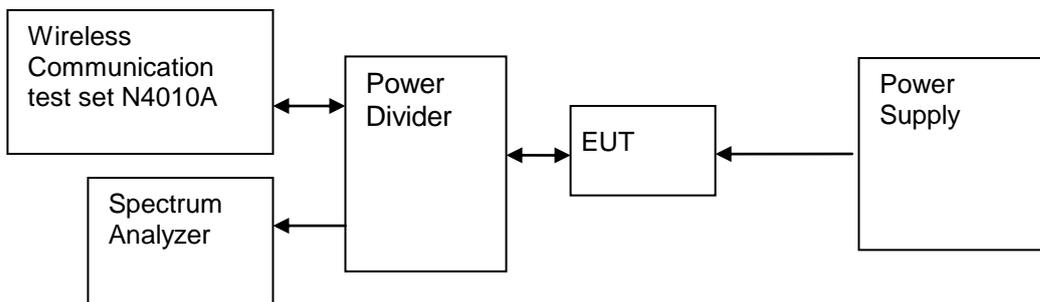
Figure 5. Test Set-up
